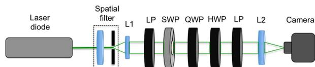
FIGURE 1. Schematic diagram employed for the experimental determination of the Spatial Average Symmetry associated to unconventional polarized beams of light. A light beam is spatially filtered and then collimated by lens L1; LP represents a linear polarizer; SWP represents the S-waveplate converter; QWP and HWP represent quarter- and half-waveplates, respectively; L2 is a lens employed to form an image on the plane of a CMOS camera.
