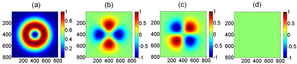
FIGURE 4. Stokes parameters associated to theoretical azimuthal polarizations, (a)  $S_0$ , (b)  $S_1$ , (c)  $S_2$ , (d)  $S_3$ . Spatial average symmetry,  $\langle S \rangle_{spa} = [1.0000 \ 0.0000 \ 0.0000 \ 0.0000]^T$ . Values are plotted in terms of pixels, and the intensity values have been normalized.
