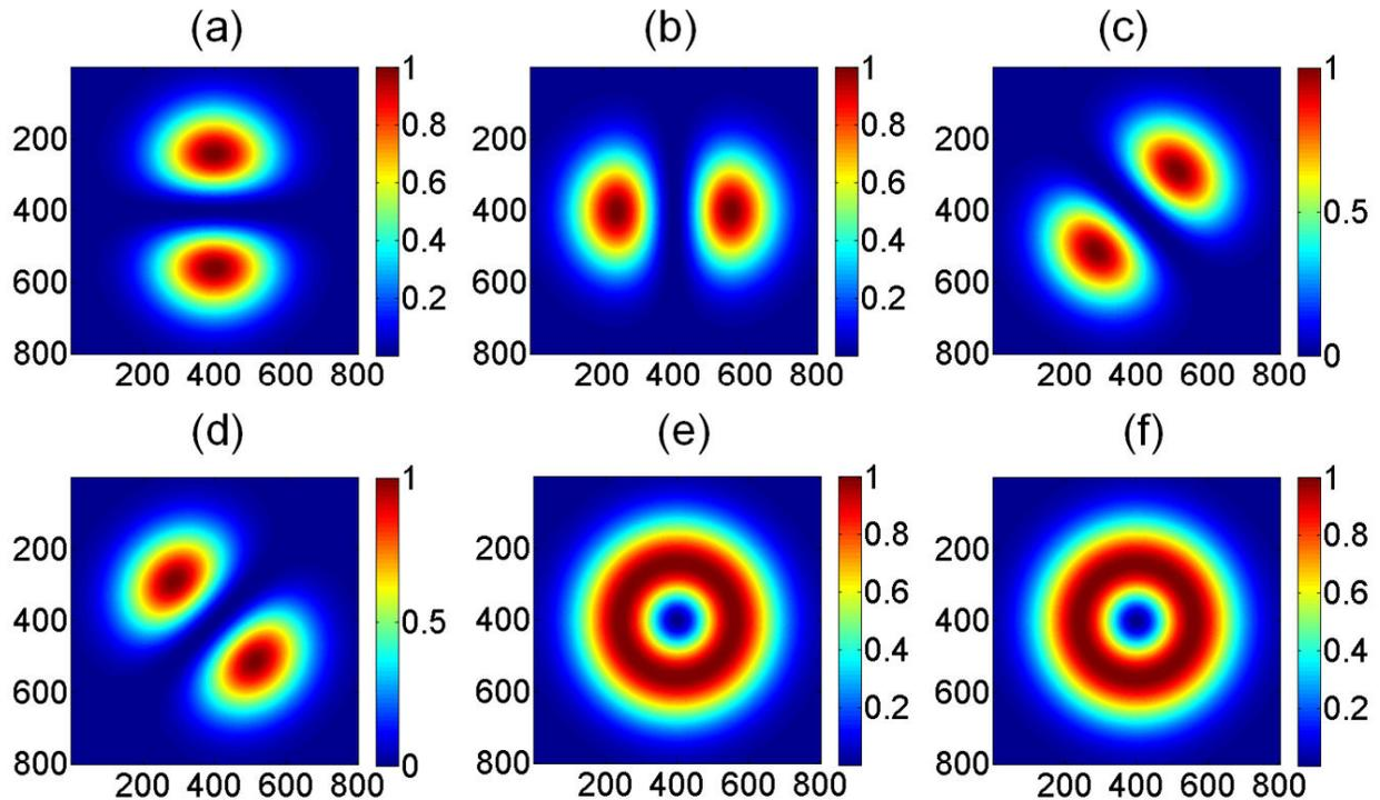
FIGURE 3. Analyzed polarization states associated to theoretical azimuthal polarization. Figs. (a), (b), (c), and (d) correspond to linear polarization states x, y,  $45^\circ$ , and  $135^\circ$ , respectively, while (e) and (f) correspond to circular right- and left-hand polarizations, respectively. Values are plotted in terms of pixels, and the intensity values have been normalized.
