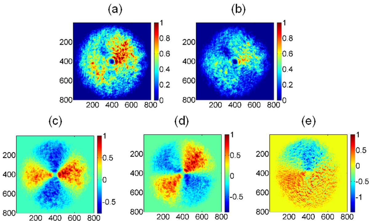
FIGURE 5. Stokes parameters associated to experimental radial polarization mode, (a) intensity spatial distribution as detected by the CMOS camera, (b)  $S_0$ , (c)  $S_1$ , (d)  $S_2$ , (e)  $S_3$ . Spatial average symmetry,  $\langle S \rangle_{spa} = [1.0000 \ 0.0851 \pm 0.0101 \ 0.1013 \pm 0.0046 \ -0.0879 \pm 0.0072]^T$ . Values are plotted in terms of pixels and the intensity values have been normalized.
