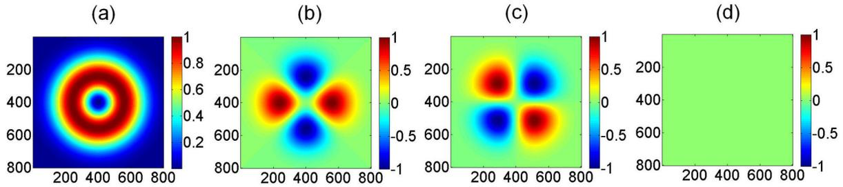
FIGURE 6. Stokes parameters associated to theoretical radial polarization, (a)  $S_0$ , (b)  $S_1$ , (c)  $S_2$ , (d)  $S_3$ . Spatial average symmetry,  $\langle S \rangle_{spa} = [1.0000 \ 0.0000 \ 0.0000 \ 0.0000]^T$ . Values are plotted in terms of pixels and the intensity values have been normalized.
