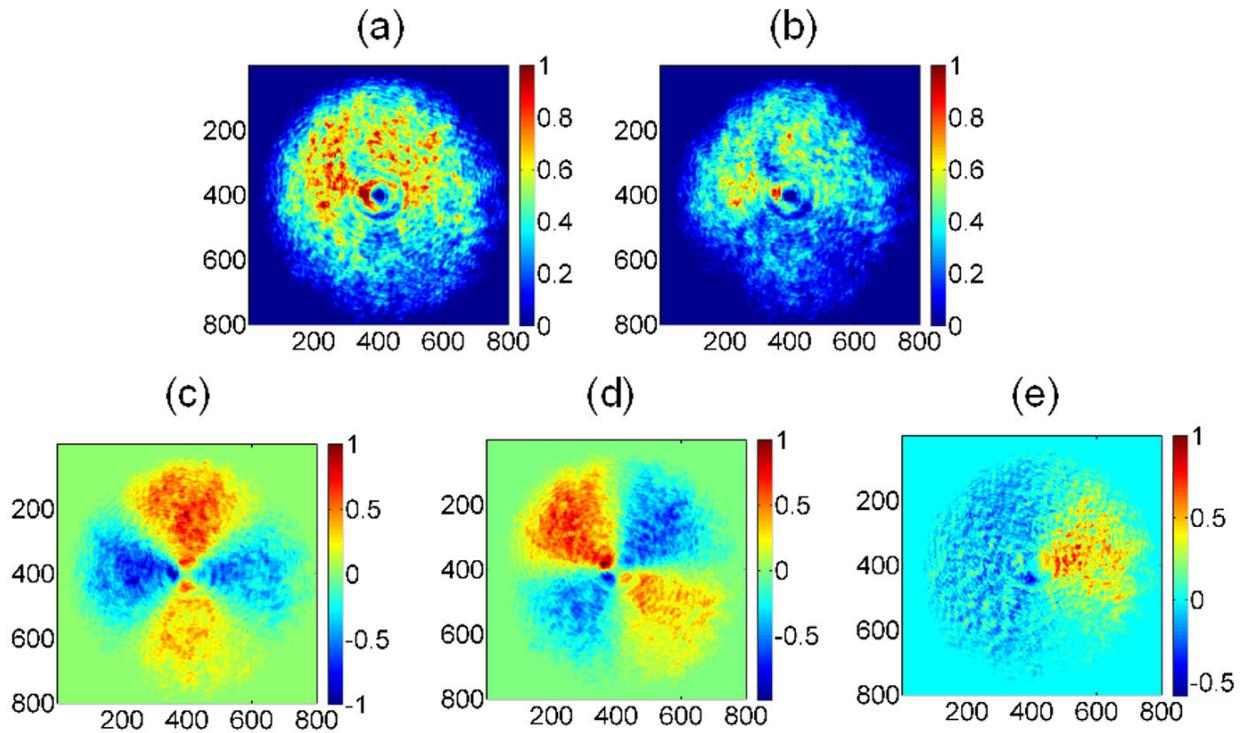
FIGURE 2. Stokes parameters associated to the experimental azimuthal polarization, (a) intensity spatial distribution as detected by the CMOS camera, (b)  $S_0$ , (c)  $S_1$ , (d)  $S_2$ , (e)  $S_3$ . Spatial average symmetry,  $\langle S \rangle_{\text{spa}} = [1.0000 \quad 0.0005 \pm 0.0022 \quad 0.0282 \pm 0.0055 \quad 0.1528 \pm 0.0048]^T$ . Values are plotted in terms of pixels, and the intensity values have been normalized.
