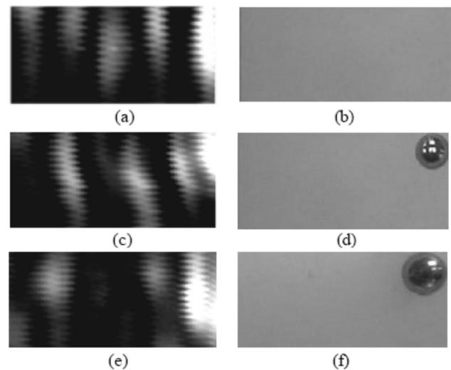
FIGURE 4. Gray-scale near-field images of  $4 \times 8 \text{ cm}^2$  due to the elasti scattering of an evanescent microwave mode travelling from left to right on the wax surface prism (a,c,e), and corresponding surface digital picture showing a sphere of radius of 0 (b), 1.5 (d) and 3 (f) cm. Scale bar for near field images is the same as in Fig. 3.
