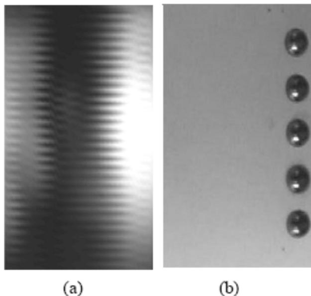
FIGURE 5. Gray-scale near-field image of  $4.5 \times 10 \text{ cm}^2$  due to the elastic scattering of an evanescent microwave mode travelling from left to right on the line of scatterers placed along the wax surface prism (a), and corresponding surface digital picture. Scale bar for the near field image is the same as in Fig. 3.
