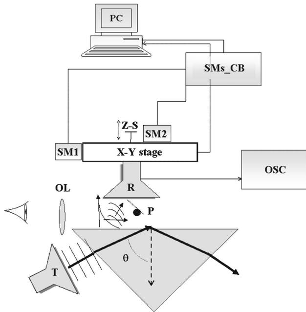
FIGURE 1. Diagram of the scanning near-field microwave microscope for imaging intensity distributions of evanescent modes generated at wavelength  $\lambda = 2.85$  cm. T, Transmitter;  $\theta$ , Incidence Angle; OL, Optical Lens; P, Signal Probe; R, Receptor; OSC, Digital Oscilloscope; SMs\_CB, Step-Motors Controller Board; PC, Personal Computer; SM1, SM2, Step-Motors 1,2; Z-S, Screw for z-motion.
