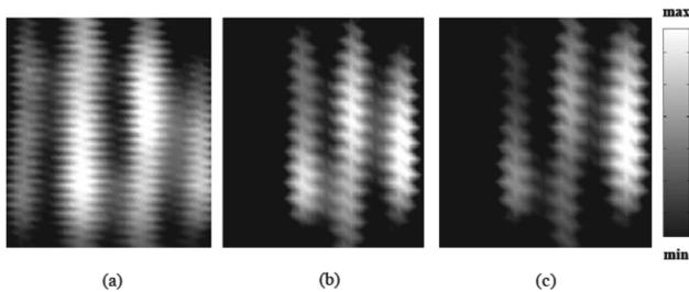
FIGURE 3. Gray-scale near-field images of  $4 \times 4 \text{ cm}^2$  generated due to the standing evanescent wave at the surface on the base of the wax prism. The images were taken at the same place for different probe-to-surface distances:  $\sim 0$  (a), 2 (b), and  $\sim 10$  mm (c).
