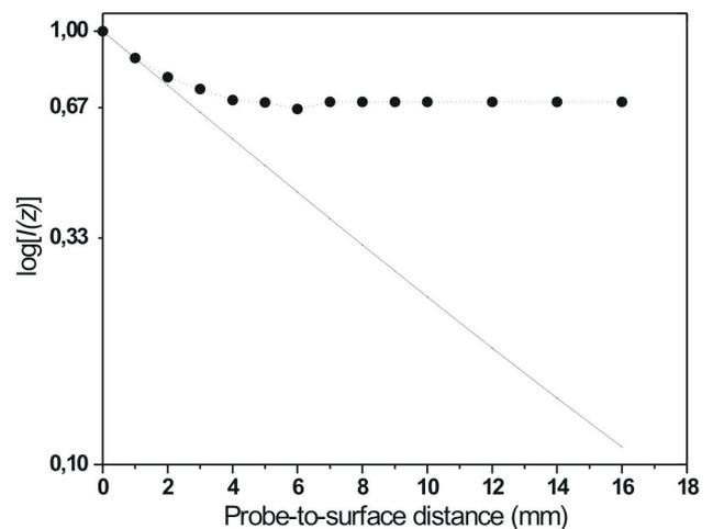
FIGURE 2. Calculated (solid line) and measured probe-to-surface distance dependence of the signal for the wax prism. Dashed line connecting the experimental points serve to guide the eye.
