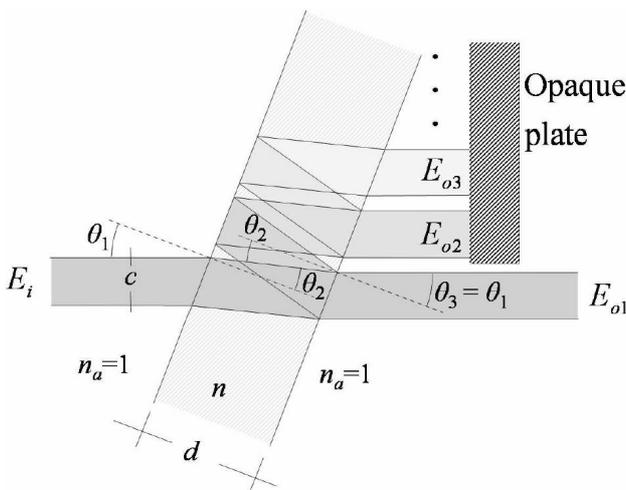
FIGURE 3. Transmission through a glass plate ( $n_a = 1$  and  $n = 1.5$ ).
