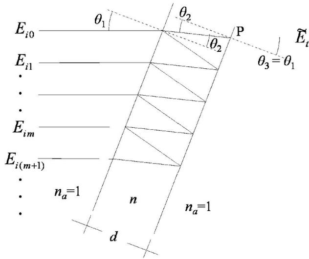
FIGURE 4. Several points from the incident wavefront contribute to the output wavefront at point P.
