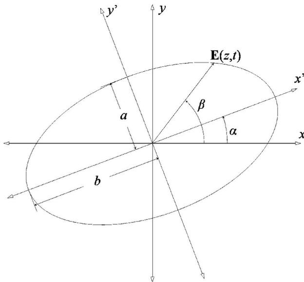
FIGURE 1. Electric wave elliptically polarized.
