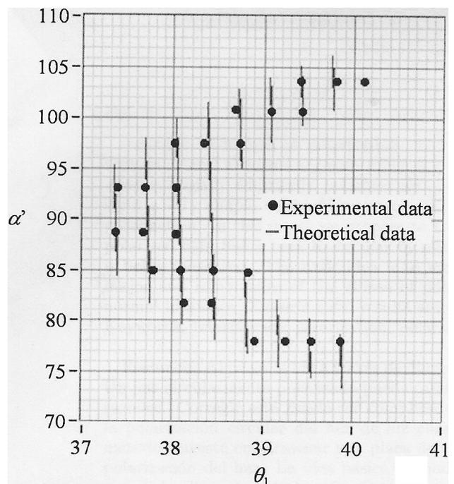
FIGURE 7. Experimental solutions (dots) vs. theoretical ones (continued) for  $e \geq 0.995$ , it means  $e=1$  in the PA410 polarimeter.
