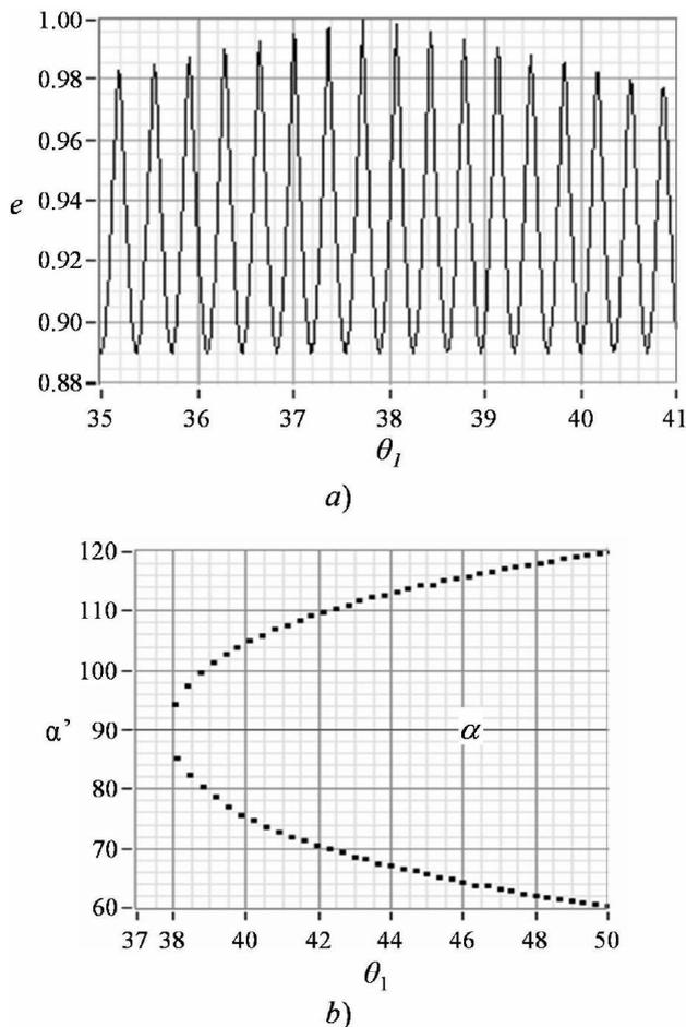
FIGURE 6. a) Ellipticity  $e$  vs. angle of incidence  $\theta_1$  with  $\alpha' = \alpha$ , and b) Solutions  $\alpha', \theta_1$  where  $e \cong 1$ .
