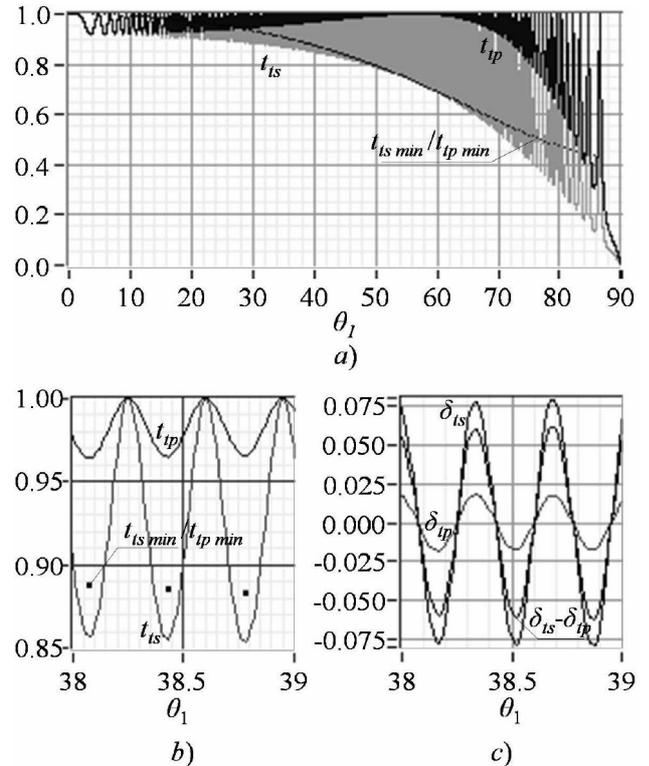
FIGURE 5. a) Theoretical total transmittances vs. angle of incidence (in deg) for a plate  $n=1.5239$ ,  $d=147\mu$  and  $\lambda=632.8\text{nm}$ . b) Detail and c) total phase change introduced by the plate (in radians) vs. angle of incidence (in deg).
