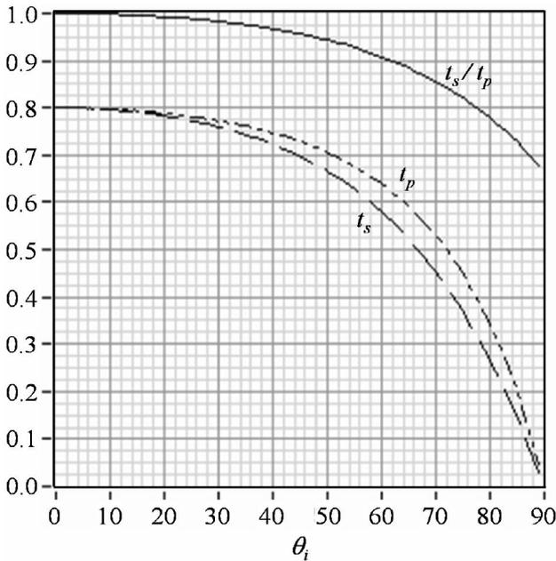
FIGURE 2. Amplitude transmittance coefficients for an air-glass interface ( $n_i = n_a = 1$  and  $n_t = n = 1.5$ ).
