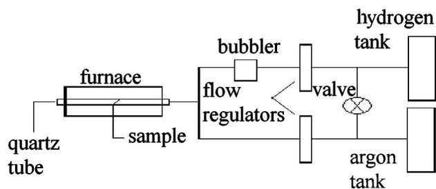
FIGURE 1. Schematic diagram of the CVD system.
