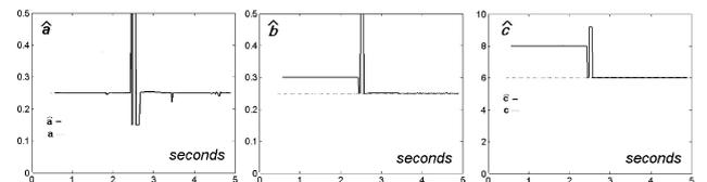
FIGURE 7. Estimation of the parameter set when an abrupt variation is introduced in the model.
