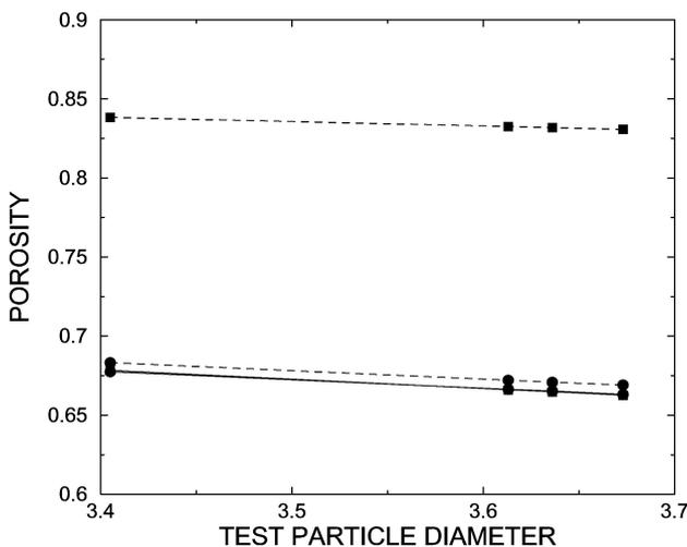
FIGURE 3. Matrix porosity as a function of the test particle diameter ( $\sigma_t$  in Å) at  $T^* = 1.5$  (solid lines) and  $T^* = 0.8$  (dashed lines) prepared with (circle) and without (square) a template. The symbols at  $T^* = 1.5$  overlap. The lines are just given as a guide.
