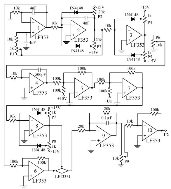
FIGURE 7. Detailed diagram of the cosine converter.
