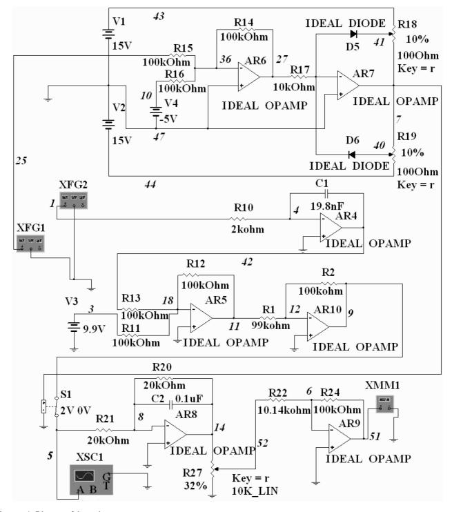
FIGURE 4. Diagram of the cosine converter.
