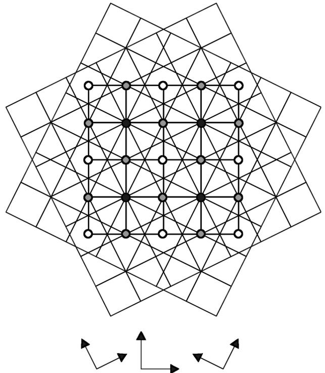
FIGURE 1. Two identical square lattices rotated 36.9 degrees with respect to each other ( $\Sigma 5$ ). The corresponding O-lattice is also displayed with shaded circles. Each shade corresponds to a set of internal coordinates, black= $\{0, 0\}$  CSL), grey= $\{0, 1/2\}$ , white= $\{1/2, 1/2\}$ . The basis vectors for  $L_1, L_2$  and the O-lattice are shown.
