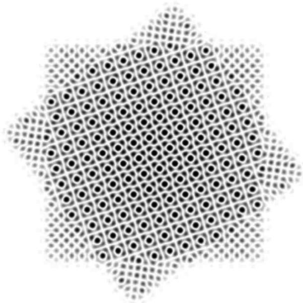
FIGURE 3. Multislice simulation (shown in reversed contrast) of two identical square lattices rotated  $36.9^\circ$  with respect to each other ( $\Sigma 5$ ). The dark wide spots mark the positions of O-lattice points.
