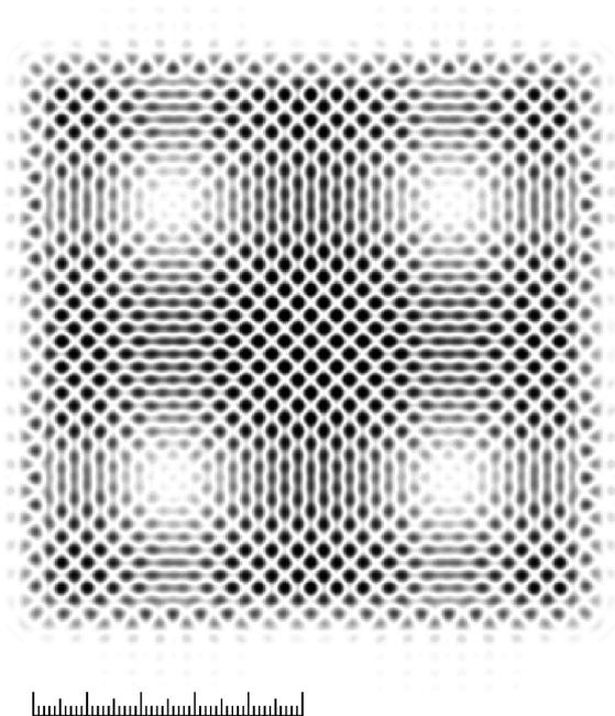
FIGURE 4. Multislice simulation of two parallel square lattices with lattice parameters differing by 10 per cent. An annular aperture was used (the contrast has been reversed for purposes of clarity).
