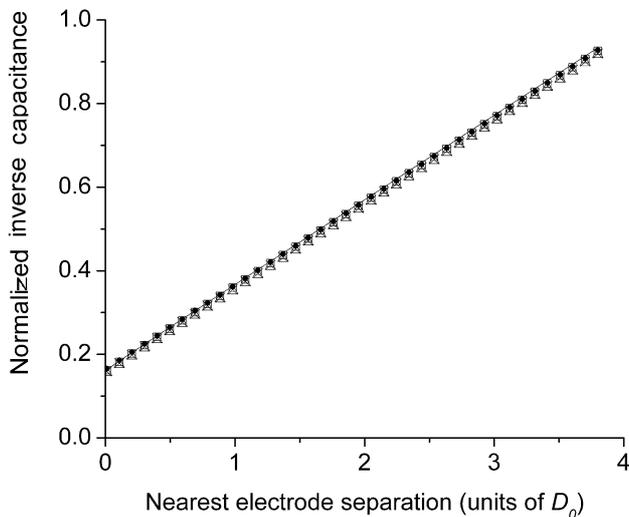
FIGURE 8. Graph of normalized capacitance against nearest electrode separation for different values of the parameter  $b$  for a band-limited fractal surface with  $\sigma = 0.2D_0$  and  $D = 1.5$ . The crosses are for the case of  $b = 1.02$ ; continuous line,  $b = 1.2$ ; open squares,  $b = 1.5$ ; filled circles,  $b = 2.0$ ; and open triangles,  $b = 2.5$ .
