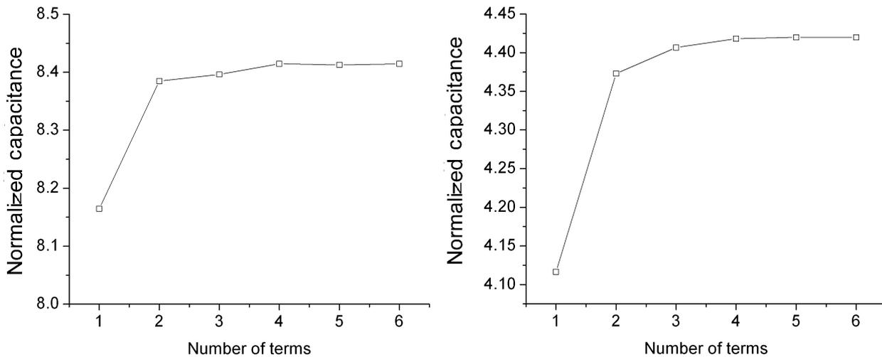
FIGURE 7. Graphs of normalized capacitance against the number,  $N$ , of spatial frequency components used in the surface generation for  $\sigma = 0.2D_0$ , left, and  $\sigma = 0.4D_0$ , right. The correlation distance for the cases shown is  $\tau = 5D_0$ .
