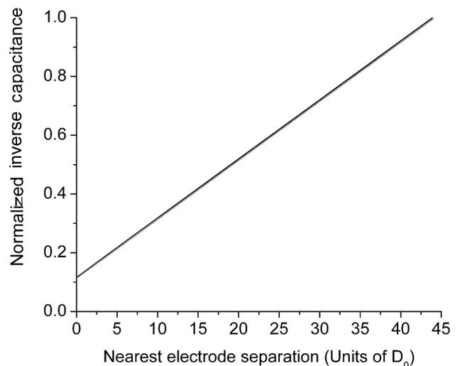
FIGURE 6. Graph of inverse normalized capacitance against nearest electrode separation for a band-limited fractal surface with  $\sigma = 0.2D_0$  and a correlation length varying from 1.0 to 6.0. In this graph there are 7 different curves, which are indistinguishable.
