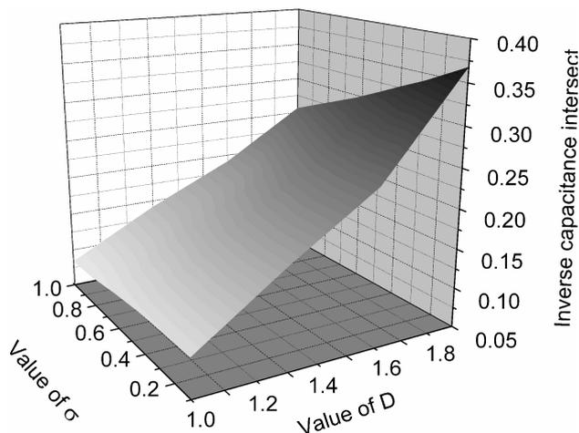
FIGURE 9. The calibration graph for the inverse capacitance intersect versus  $\sigma$  and  $D$ . The intersection of the plane for a measured value of the inverse capacitance with this curve gives the possible values of  $\sigma$  and  $D$  for the surface.
