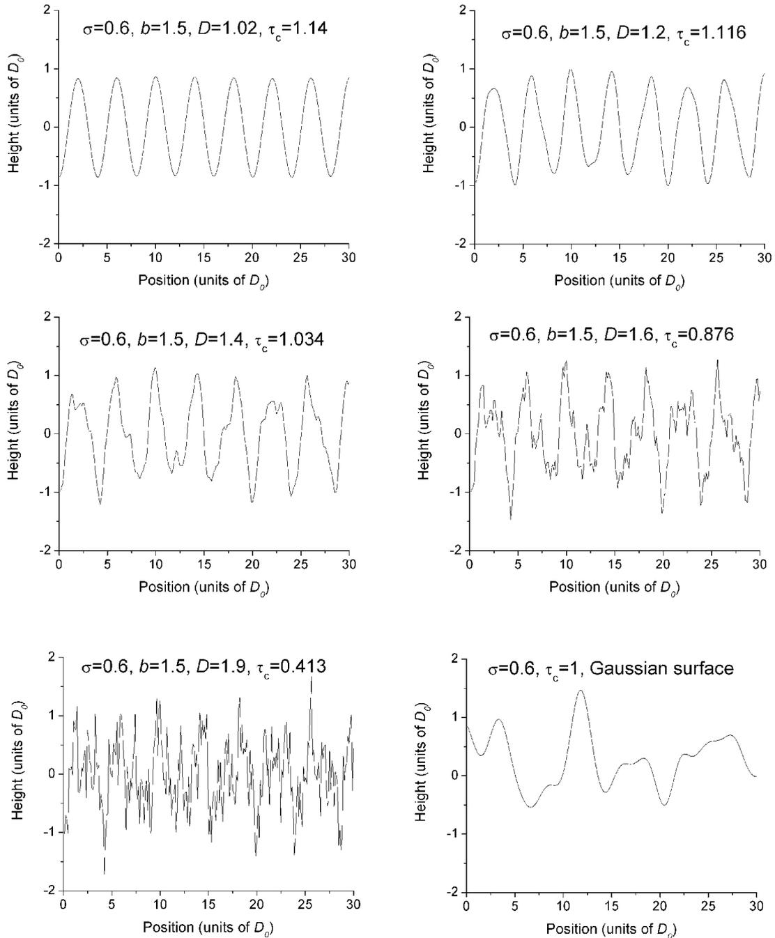
FIGURE 1. Examples of the band-limited fractal rough surface profiles and the parameters of the surfaces. Also shown for comparison is a Gaussian random rough surface with the same standard deviation of height and a correlation length comparable with the band-limited fractal surfaces.
