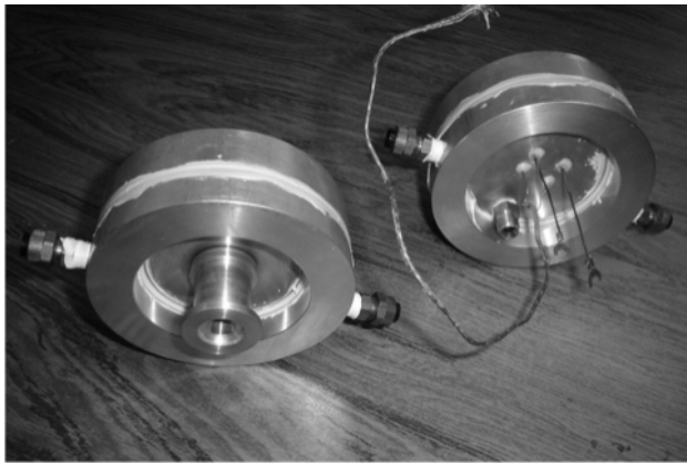
FIGURE 2. Water cooled lids designed to seal the ends of the oven. Electrical feedthroughs and vacuum pump connection are shown.
