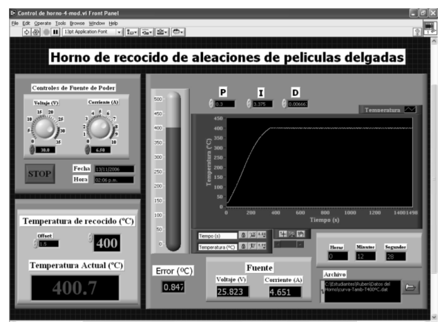
FIGURE 4. Front panel designed in LabView for the control of the vacuum oven. The heating temperature in real time of the vacuum oven can be observed.
