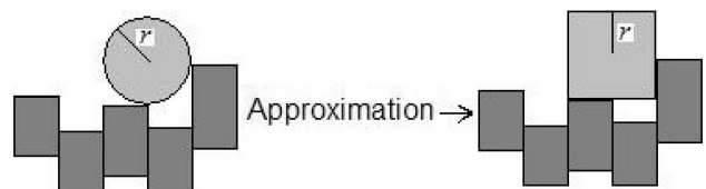
FIGURE 7. Schematic representation of the approximation used to determine if a particle penetrates the membrane.
