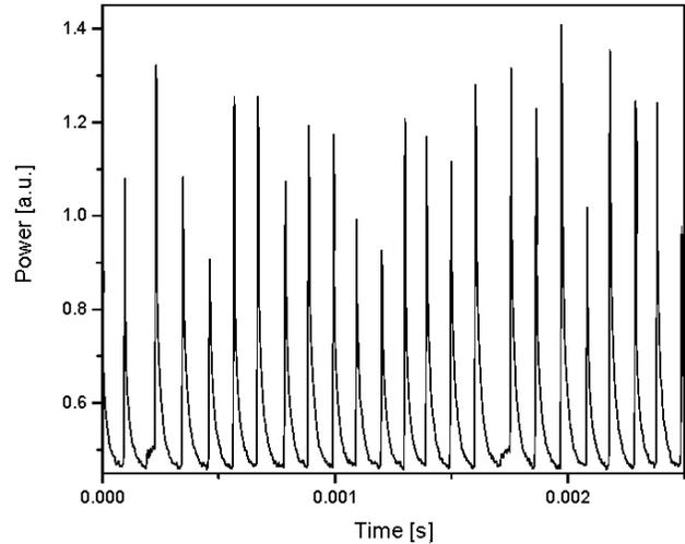
FIGURE 3. Snapshot of a pulse train of the Q-switched fiber laser at 1.7 W of launched pump power.
