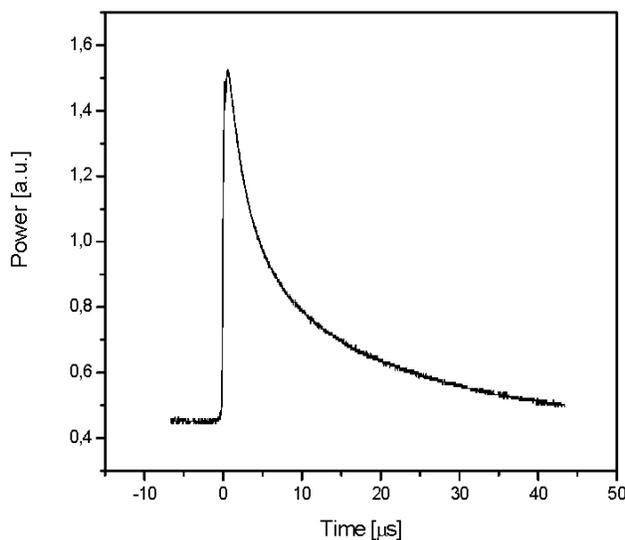
FIGURE 5. Pulse shape at 1.7 W of launched pump power.
