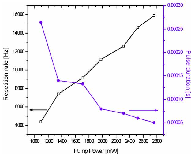
FIGURE 4. Repetition rate and pulse duration versus launched pump power.
