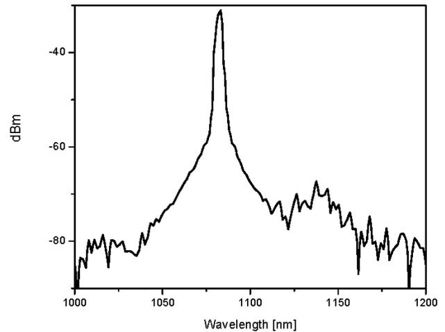
FIGURE 6. Optical spectrum of the pulsed fiber laser.
