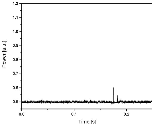
FIGURE 2. Temporal response of the fiber laser in CW regime.
