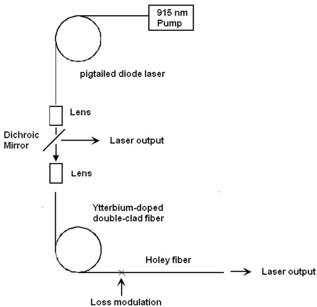
FIGURE 1. Schematic diagram of the Q-switched fiber laser setup.
