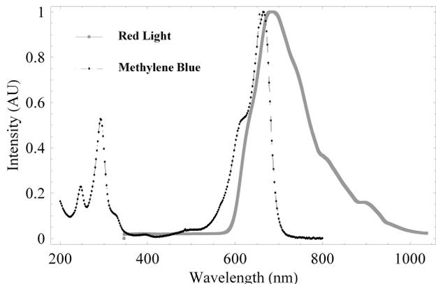
FIGURE 2. Absorption spectrum of methylene blue and optical spectrum of the light source used for this bonding agent.
