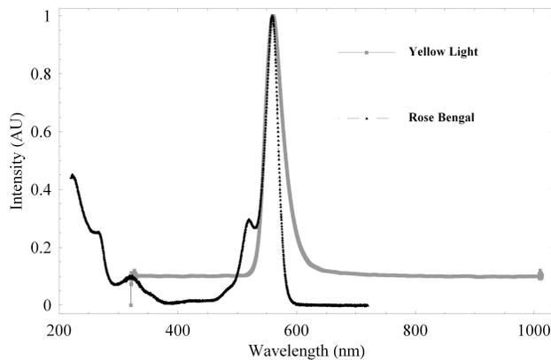
FIGURE 3. Absorption spectrum of rose bengal and optical spectrum of the light source used for this bonding agent.
