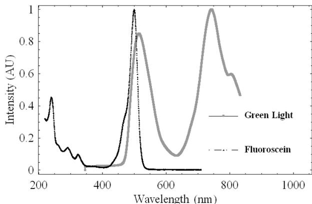
FIGURE 1. Absorption spectrum of flosorsein and optical spectrum of the light source used for this bonding agent.
