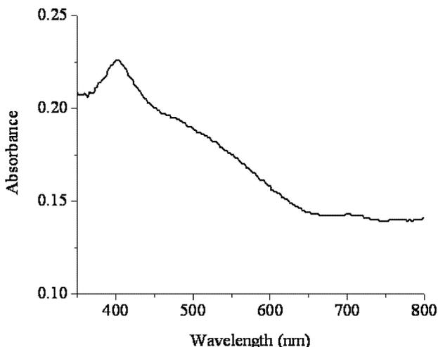
FIGURE 6. UV-vis spectra of RED-H in the solid state.
