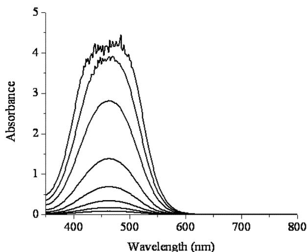
FIGURE 3. UV-vis spectra of RED-H in methanol at different concentrations. From top to bottom: a)  $2.5 \times 10^{-4}$  M, b)  $1.87 \times 10^{-4}$  M, c)  $1.25 \times 10^{-4}$  M, d)  $7.5 \times 10^{-5}$  M, e)  $3.75 \times 10^{-5}$  M, f)  $1.82 \times 10^{-5}$  M, g)  $0.93 \times 10^{-5}$  M, h)  $0.46 \times 10^{-5}$  M.
