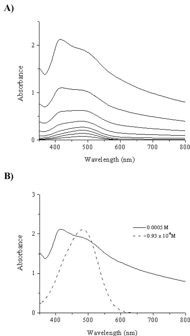
FIGURE 4. UV-vis spectra of RED-H in methanol: water 40:60. **A)** at different concentrations. From top to bottom: a) 0.0005 M, b)  $2.5 \times 10^{-4}$  M, c)  $1.87 \times 10^{-4}$  M, d)  $1.25 \times 10^{-4}$  M, e)  $7.5 \times 10^{-5}$  M, f)  $3.75 \times 10^{-5}$  M, g)  $1.82 \times 10^{-5}$  M, h)  $0.93 \times 10^{-5}$  M, i)  $0.46 \times 10^{-5}$  M. **B)** at 0.0005 M and  $0.93 \times 10^{-5}$  M (normalized spectra).
