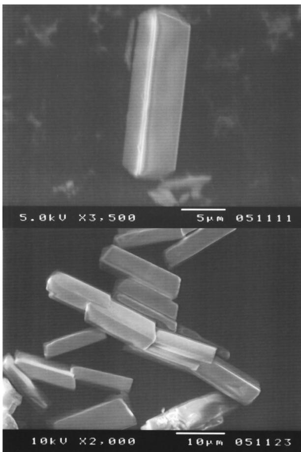
FIGURE 6. SEM micrographs of a single particle and a first-order agglomerate of polycrystalline particles. These were produced guided by an applied magnetic field.
