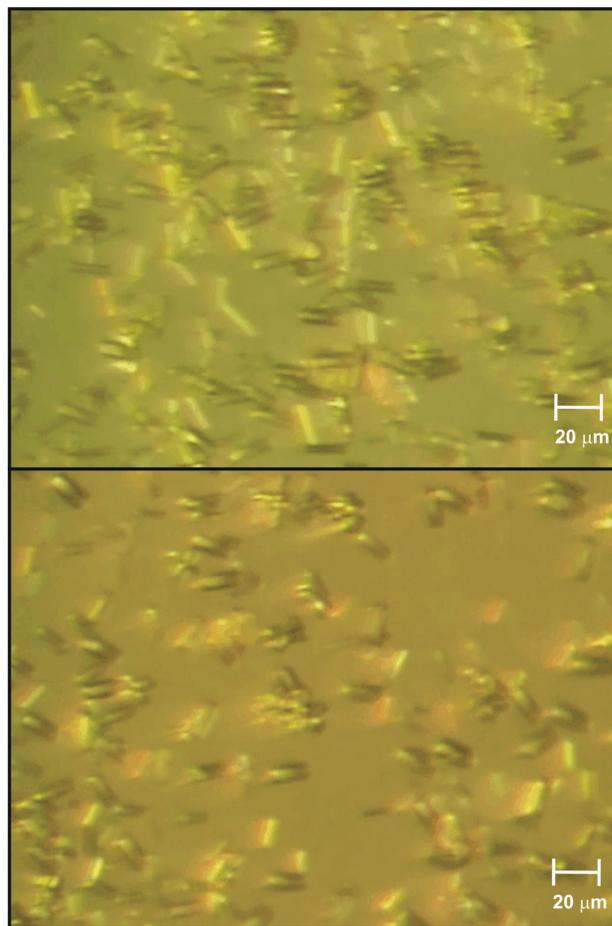
FIGURE 1. Microphotographs of the distribution of particles of iron oxalate at the end of the coprecipitation reaction. pH = 1.2 upper and 5.4 lower.
