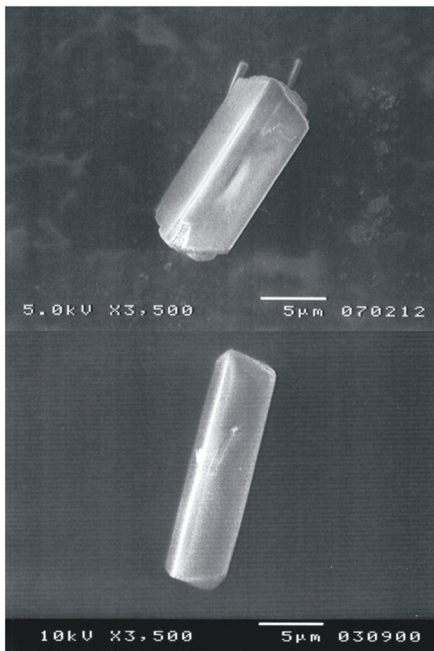
FIGURE 2. SEM micrographs of prismatic polycrystalline particles of iron oxalate obtained by aggregation of crystallites during a precipitation process, for two different pH values, upper pH = 1.2 and lower pH = 5.4.
