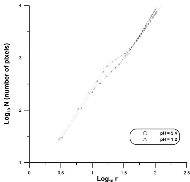
FIGURE 3.  $\log_{10} N$  vs  $\log_{10} r$  for the final structures formed by the polycrystalline particles obtained by the coprecipitation process at different pH conditions. The values of  $r$  are expressed in terms of the particle mean size  $\sigma$ .
