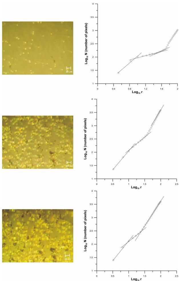
FIGURE 5. Microparticles distribution during the coprecipitation process at pH =5.4 and with an applied static magnetic field ( $H = 0.022T$ ). The photographs show the beginning (upper), a middle stage and the final of the process (lower). The corresponding graph of  $\log_{10}N$  vs  $\log_{10}r$  is shown next in the right.
