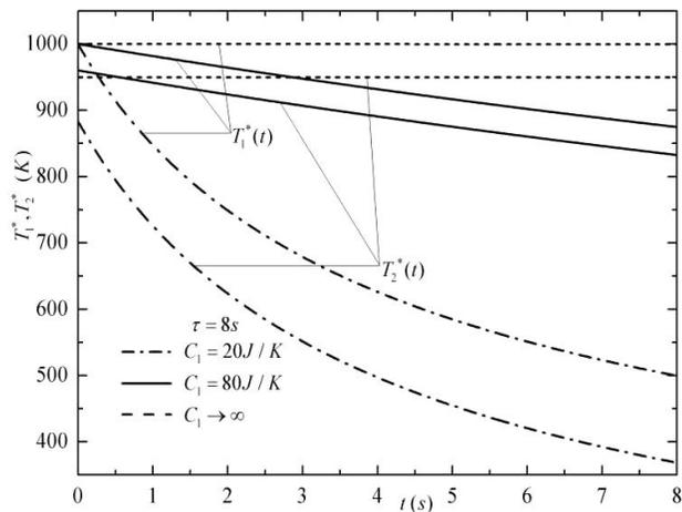
FIGURE 8. Optimal temperature configurations for the finite-time exergy during the heat transfer processes with the radiative heat transfer law.
