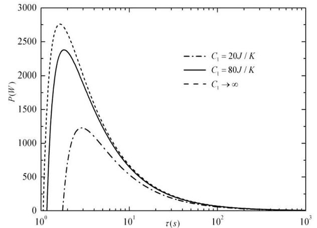
FIGURE 4. Maximum average power versus process duration for the case with Newton's heat transfer law.
