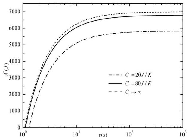
FIGURE 6. Finite-time exergy versus process duration for the case with the linear phenomenological heat transfer law.
