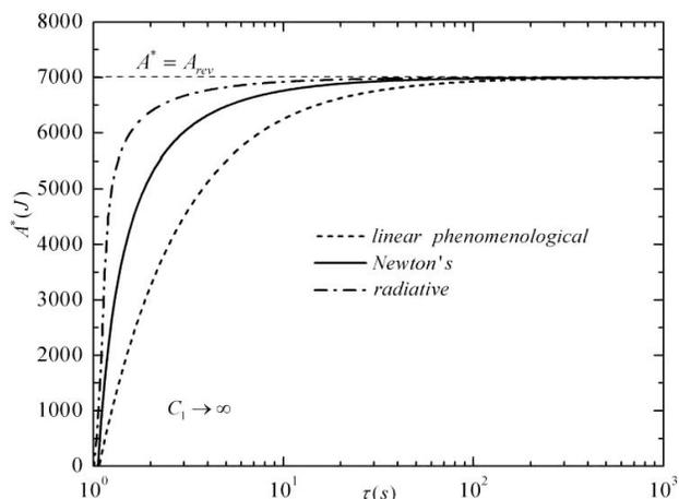
FIGURE 10. Finite-time exergy versus process duration for the cases with different heat transfer laws.
