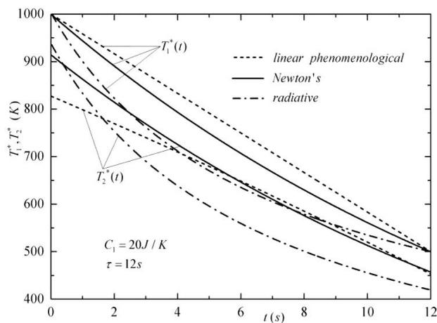
FIGURE 9. Optimal temperature configurations for the finite-time exergy during the heat transfer processes with different heat transfer laws.
