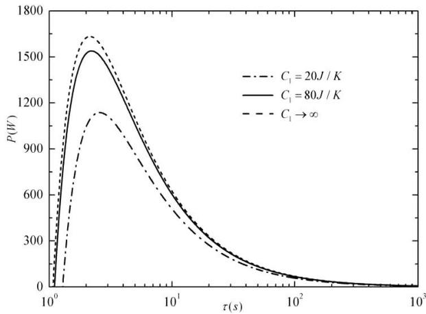
FIGURE 7. Maximum average power versus process duration for the case with the linear phenomenological heat transfer law.
