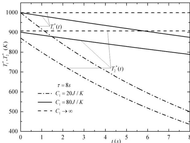
FIGURE 2. Optimal temperature configurations for the finite-time exergy during the heat transfer processes with Newton's heat transfer law.
