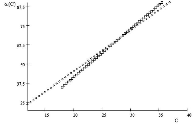
FIGURE 1. Plot of the friction factor  $\alpha$  as a function of the compactness  $C$  for elliptic ( $\circ$ ) and rectangular ( $\square$ ) cross-sections.
