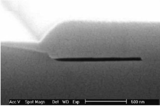
FIGURE 2. Scanning by SEM of the cross-section of a nano-channel [4]. The black zone at the middle part has a size  $w=900$  nm and height  $h = 50$  nm.
