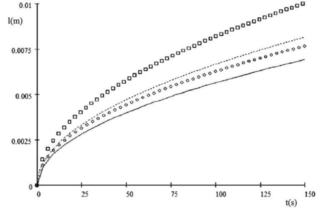
FIGURE 3. Plot of  $l$  vs  $t$ : continuous line corresponds to the Washburn law using the hydraulic radius  $R_H$  (Eq. (32));  $\square$  experimental data from Han *et al* [4];  $\circ$  elliptic cross-section using Eq. (28) and dashed line rectangular nano-channel with  $w = 900$  nm and height  $h = 50$  nm Eq. (31).
