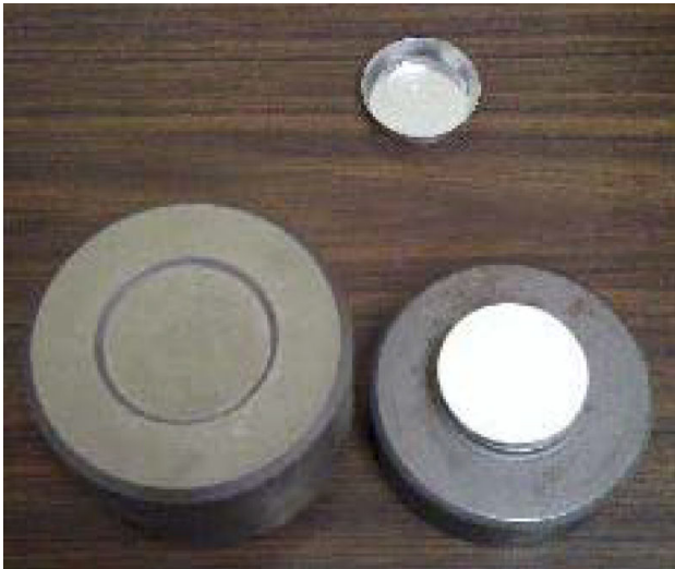
FIGURE 1. Aluminum container and final 40 K standard
