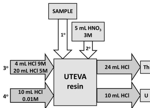
FIGURE 3. Chromatographic separation technique using UTEVA resin.
