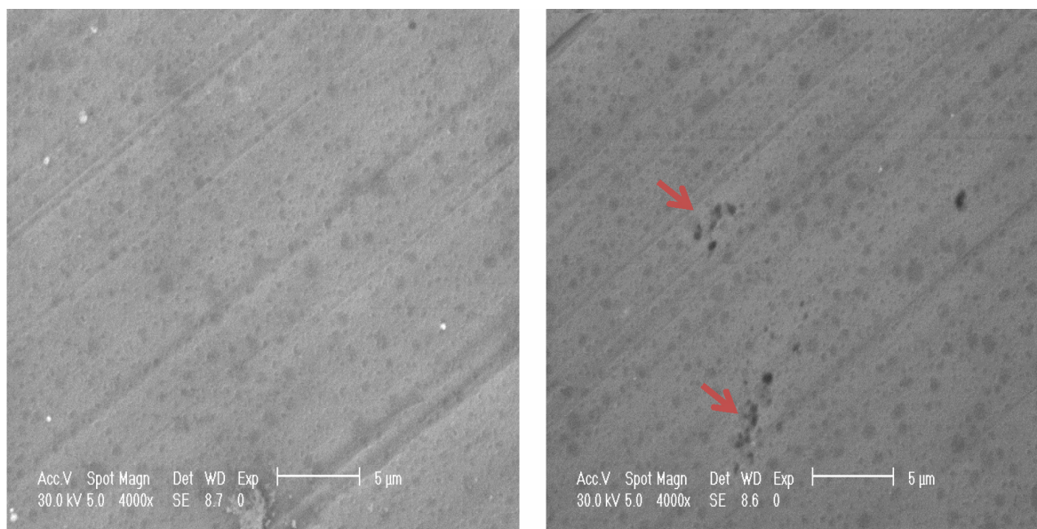
FIGURE 7. a) SEM micrograph the morphology of ZrN_xO_y thin film before polarization. b) after polarization in NaCl 3,5%, deposited at 350 W, 623 K and flow ratio of 1.25. Steel 316L coated with ZrN_xO_y film.
