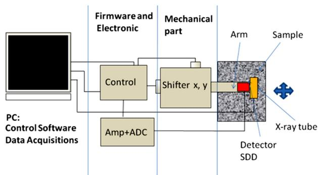
FIGURE 1. Experimental setup for the XRF Imaging System.
