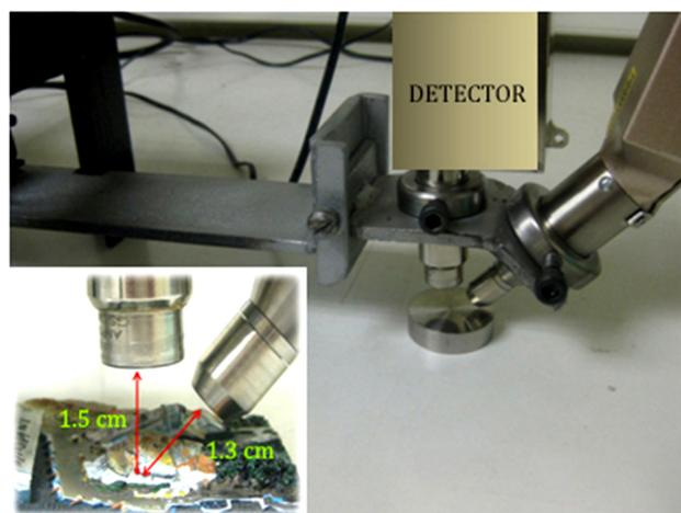
FIGURE 2. Robotic arm. It is shown MTRX-sample and sample-SDD distances.
