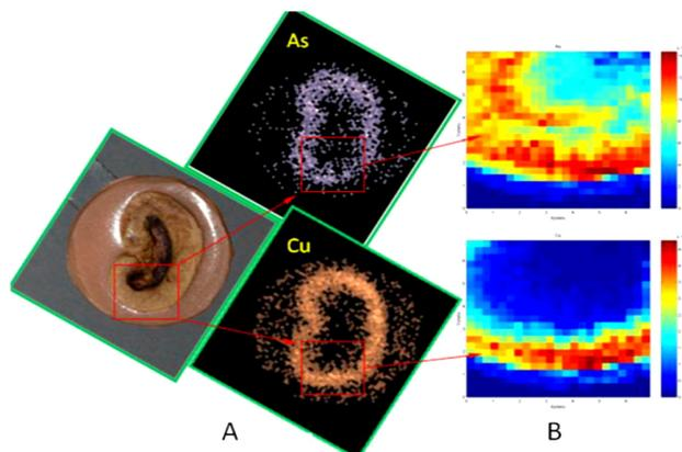
FIGURE 4. Multi-elemental XRF images of As-exposed rat kidney. Images obtained by 2D rapid EDXRF device, counting time 30 ms/pixel ( $200 \times 200 \mu\text{m}$ ), total acquisition time 22 min (A). Images obtained by SR- $\mu$ XRF, counting time 10 s/pixel ( $200 \times 200 \mu\text{m}$ ), total acquisition time 1.47 h (B).
