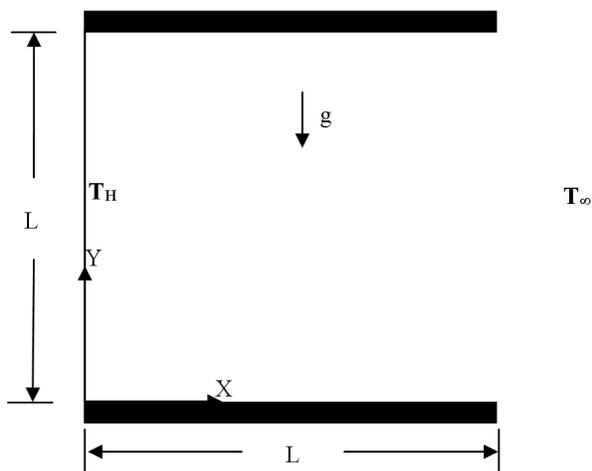
FIGURE 1. Scheme of the physical model.
