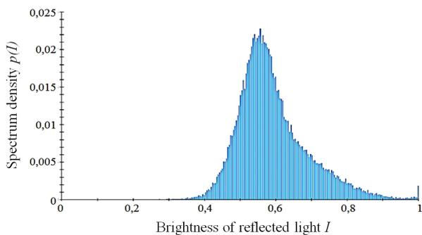
FIGURE 1. Brightness spectrum of the visible light reflections from the surface of one specimen fragment before fatigue testing.
