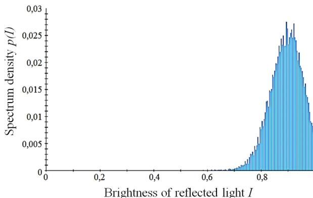
FIGURE 3. Range of reflected light brightness of the fragment of Figure 1 after the specimen experienced fatigue crack in a test.
