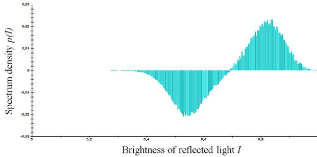
FIGURE 5. Difference in the brightness spectra of the visible light reflections from a fragment's surface (Specimen No. 1).
