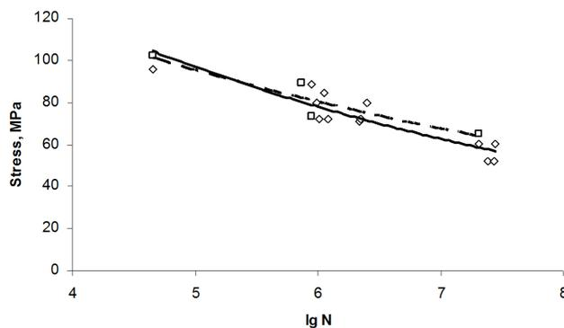
FIGURE 6. Fatigue curves for aluminum alloy 2024 (Obtained from the D16 Russian standard), constructed according to the data of standard tests ( $\square$ ) and by photometric analysis of the specimens' surfaces ( $\diamond$ ).
