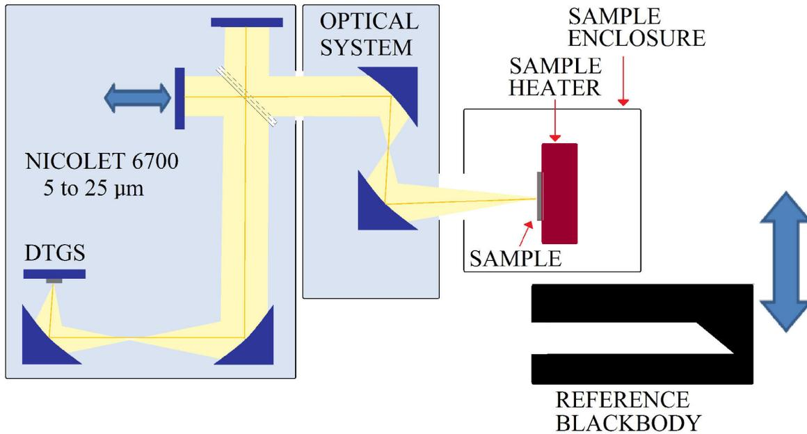
FIGURE 1. Experimental setup for emissivity measurement at CENAM.
