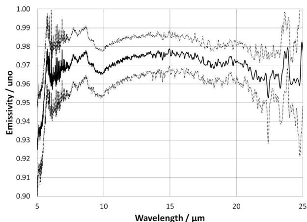
FIGURE 2. Spectral emissivity and uncertainty of high-emissivity black paint in the range from 5 to 25 micrometers.
