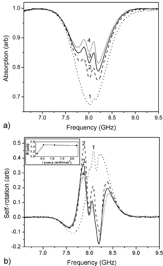
FIGURE 7. Absorption (a) and self-rotation (b) curves for a co-propagating beam in transition  $F_g = 1, F_e = 0$ . The pump laser intensity is: Curve 1:  $0 \text{ mW/mm}^2$ , curve 2:  $0.55 \text{ mW/mm}^2$ , curve 3:  $1.11 \text{ mW/mm}^2$  and curve 4:  $2.22 \text{ mW/mm}^2$ . The signal intensity is  $2.9 \text{ mW/mm}^2$ . The variation of  $R$  with the pump beam intensity is also shown.
