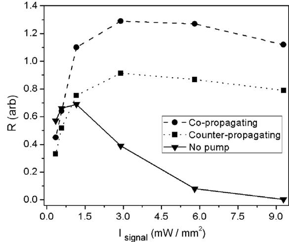
FIGURE 4. Comparative curves of  $R$  as a function of signal intensity without and with the pump beam in the transition  $F_g = 1, F_e = 0$ . The intensity of pump laser is at maximum ( $2.22 \text{ mW/mm}^2$ ).
