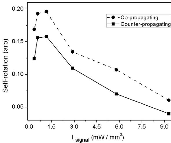
FIGURE 3. Comparative curves of self-rotation as a function of signal intensity for co- and counter-propagating pump laser in the transition  $F_g = 1, F_e = 0$ . The intensity of pump beam is at maximum ( $2.22 \text{ mW/mm}^2$ ).
