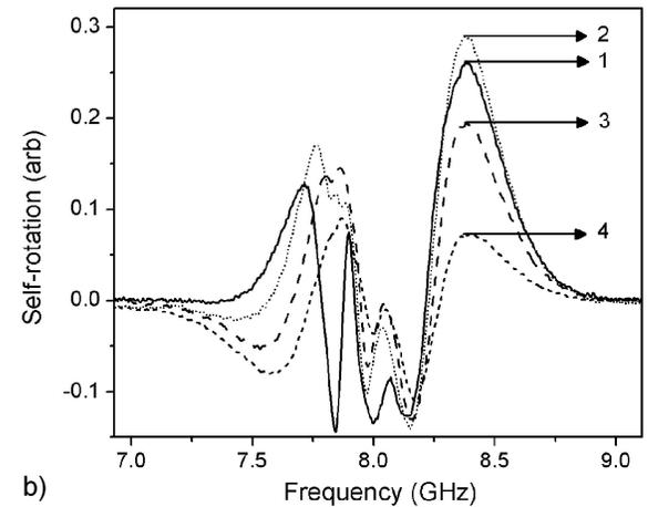
FIGURE 5. Absorption and self-rotation curves for a parallel polarization of the pump beam impinging in a counter-propagating pump beam direction. The pump laser intensity is  $2.22 \text{ mW/mm}^2$  and the signal intensity is: Curve 1:  $0.35 \text{ mW/mm}^2$ , curve 2:  $1.16 \text{ mW/mm}^2$ , curve 3:  $2.9 \text{ mW/mm}^2$  and curve 4:  $9.3 \text{ mW/mm}^2$ .
