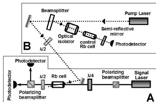
FIGURE 1. The experimental setup. The scheme marked with letter A represents the measurement arm. The scheme marked with letter B represents the pump and control arm.
