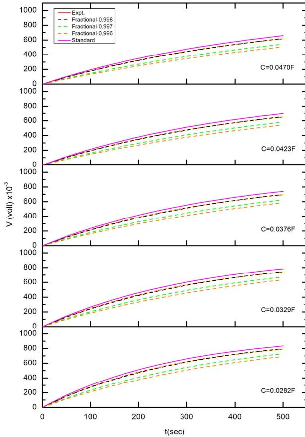
FIGURE 3. During charging a capacitor, the changing of voltage of capacitor in the course of time for  $\varepsilon = 1$  V,  $R = 10$  k $\Omega$  and different capacitors which are  $C = 0.047$  F,  $C = 0.0423$  F,  $C = 0.0376$  F,  $C = 0.0329$  and  $C = 0.0282$  F. (The error bars have been shown with yellow).
