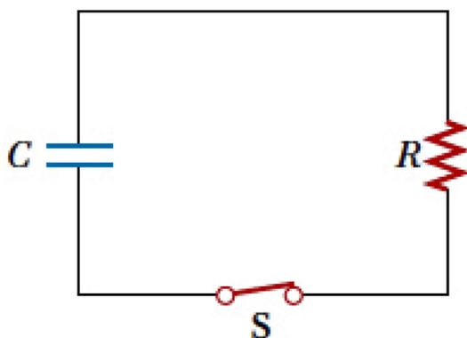
FIGURE 2. Discharging a capacitor in RC circuit.
