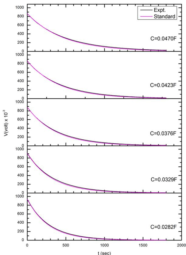
FIGURE 5. During discharging a capacitor, the changing of voltage of capacitor in the course of time for  $R = 10 \text{ k}\Omega$  and different capacitors which are  $C = 0.047 \text{ F}$ ,  $C = 0.0423 \text{ F}$ ,  $C = 0.0376 \text{ F}$ ,  $C = 0.0329$  and  $C = 0.0282 \text{ F}$ .
