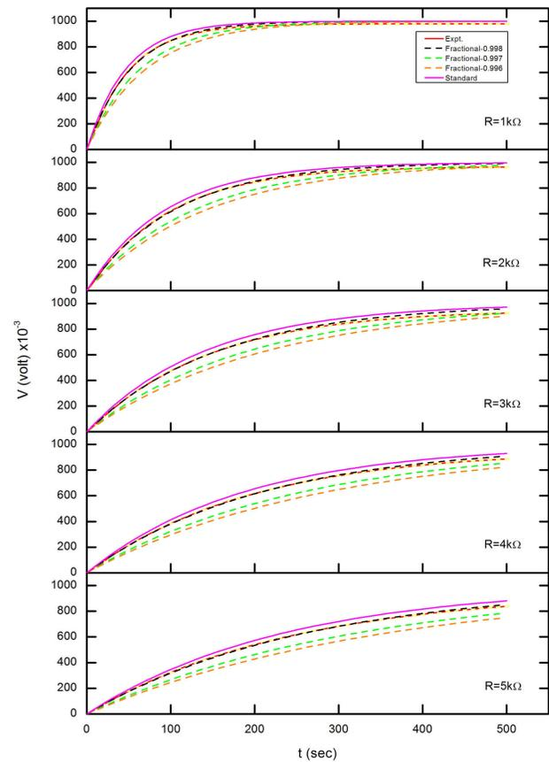
FIGURE 4. During charging a capacitor, the changing of voltage of capacitor in the course of time for  $\varepsilon = 1$  V,  $C = 0.047$  F and different resistances which are  $R = 1$  k $\Omega$ ,  $R = 2$  k $\Omega$ ,  $R = 3$  k $\Omega$ ,  $R = 4$  k $\Omega$  and  $R = 5$  k $\Omega$ . (The error bars have been shown with yellow).
