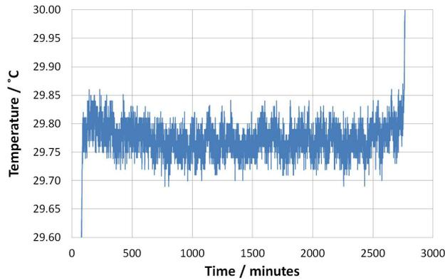
FIGURE 3. Measurement of the phase transition (fusion) of gallium with CENAM's transfer radiation thermometer.
