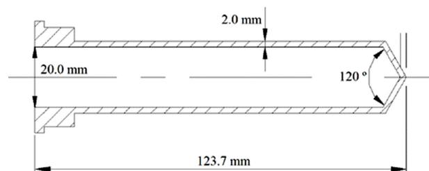
FIGURE 1. Cross-section of the blackbody cavity.
