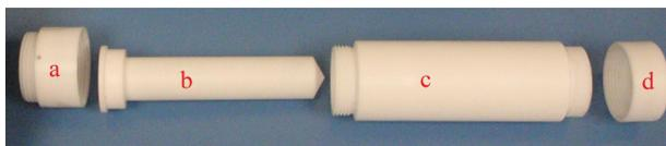
FIGURE 2. Crucible parts: (a) front cap, (b) blackbody cavity, (c) container and (d) back cap.
