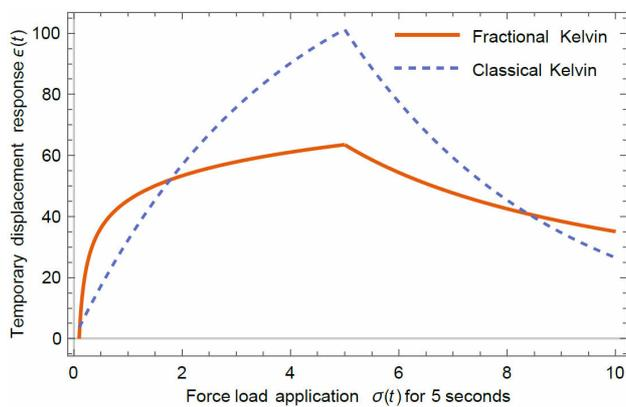
FIGURE 4. Displacement response for the Kelvin model. Fractional and integer.
