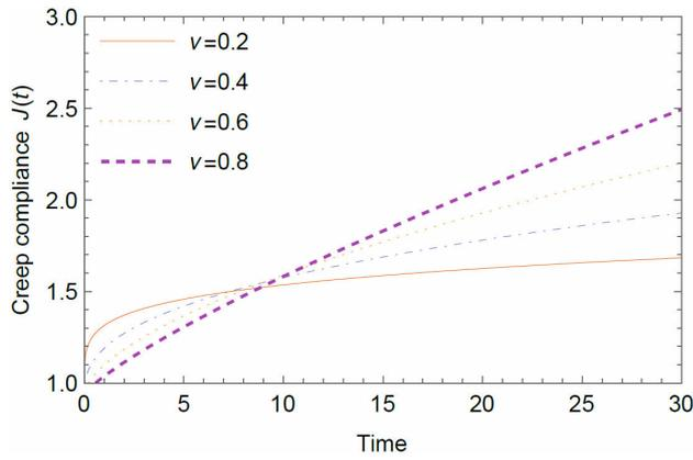
FIGURE 7. Creep compliance function, here we observe that for values close to real order  $\nu = 1$  the behavior its almost lineal.
