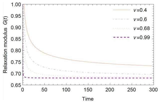
FIGURE 6. Fractional relaxation modulus, can be observed that for a near integer order,  $\nu = 0.99$  the relaxation function have an exponential behavior.
