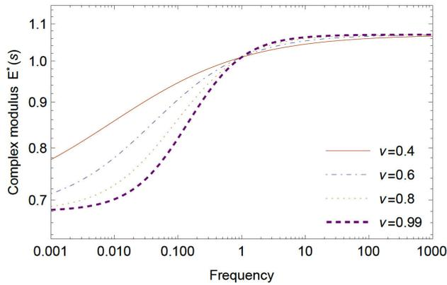
FIGURE 8. Complex modulus, observe that for values nearest to integer order one, the graphic present the traditional form.
