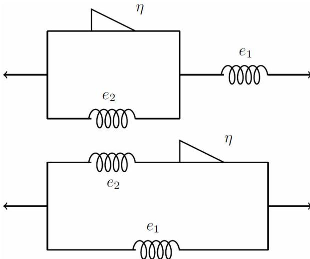
FIGURE 2. Fractional Kelvin model (FKM) on top and at the bottom Zener fractional model (FZM), can be observe that the basic idea consist in to replace the dash pot for a new element know as spring-pot.
