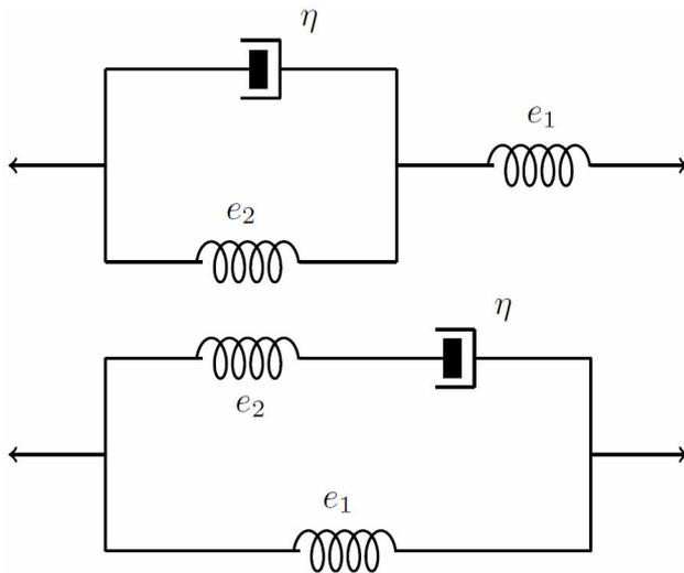
FIGURE 1. Kelvin model (KM) on top, Standard lineal solid model other known as Zener model (ZM).
