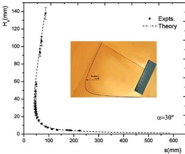
FIGURE 4. Plot of the theoretical profile (dashed lines) built with Eq. (8) and the experimental data (symbols). The picture on the inset is typical of the experimental equilibrium profiles for  $\beta = 0.523$  rad ( $30^\circ$ ) and  $\alpha = 0.0092$  rad (visible numbers are in cm scale). The error bars show a 5% error margin.
