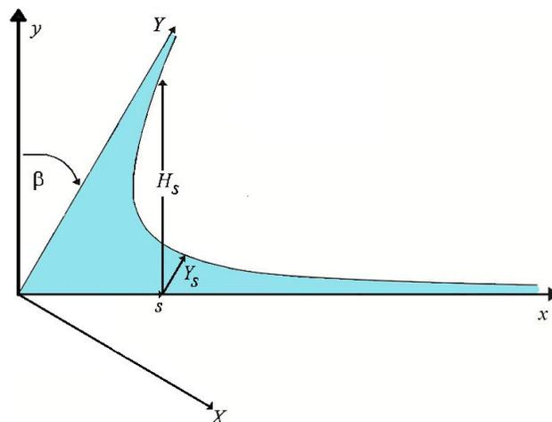
FIGURE 2. Schematic of the equilibrium profile described from the coordinate system  $(x, y)$  or from the rotated  $(X, Y)$  system. The rotation angle is  $\beta$ . In this case  $Y_s$  is the distance along the line parallel to the tilted edge and that starts at  $x = s$  and  $y = 0$ .
