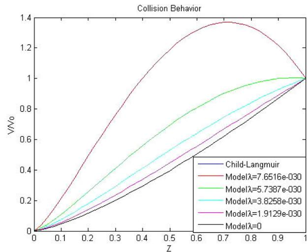
FIGURE 2. Plot showing the electrostatic potential in the adiabatic approximation with  $D = 1$ . Note how the functions for the electrostatic potential have the same value at  $z = 0$  and  $z = D$  such that the applied bias in the vacuum tube diode is  $V_0$  and when  $\lambda$  tends to zero the curves are really close to each other for  $0 < z < D$ .
