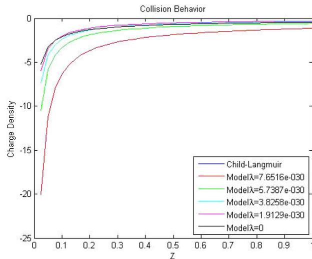
FIGURE 3. Volume charge density for our model compared to the Child-Langmuir model.
