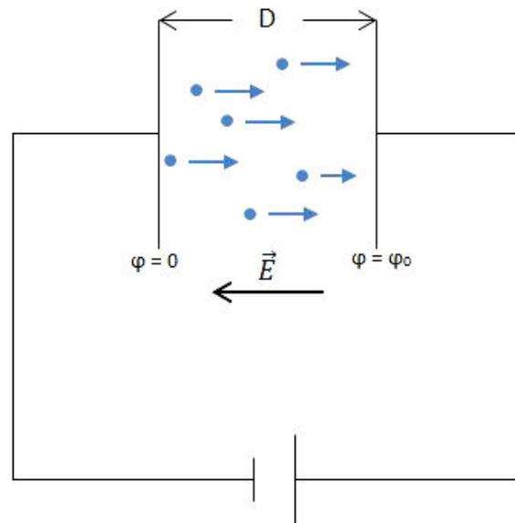
FIGURE 1. Vacuum Tube that consists of two parallel plates subjected to an electrostatic potential between its terminals. The negatively charged electrons moving to the right constitute a steady electric current.
