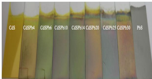
FIGURE 1. Photography of CdS0-CdSPb-PbS0 thin films.
