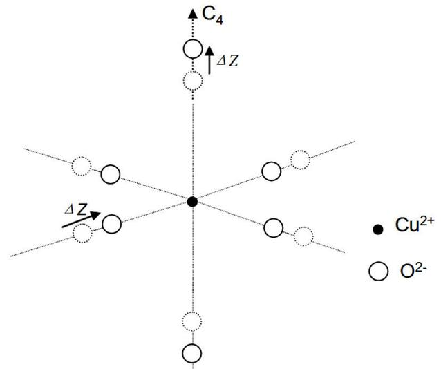
FIGURE 1. The local structure of  $\text{Cu}^{2+}$  in LiNaCdP glass.
