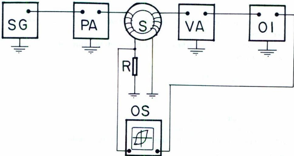
Fig. 1 Layout of the modules for the measurement of magnetic hysteresis loops. SG-signal generator, PA-power amplifier, S-sample, Va-voltage amplifier, OI-operational integrator, OS-oscilloscope, R-series resistor.
