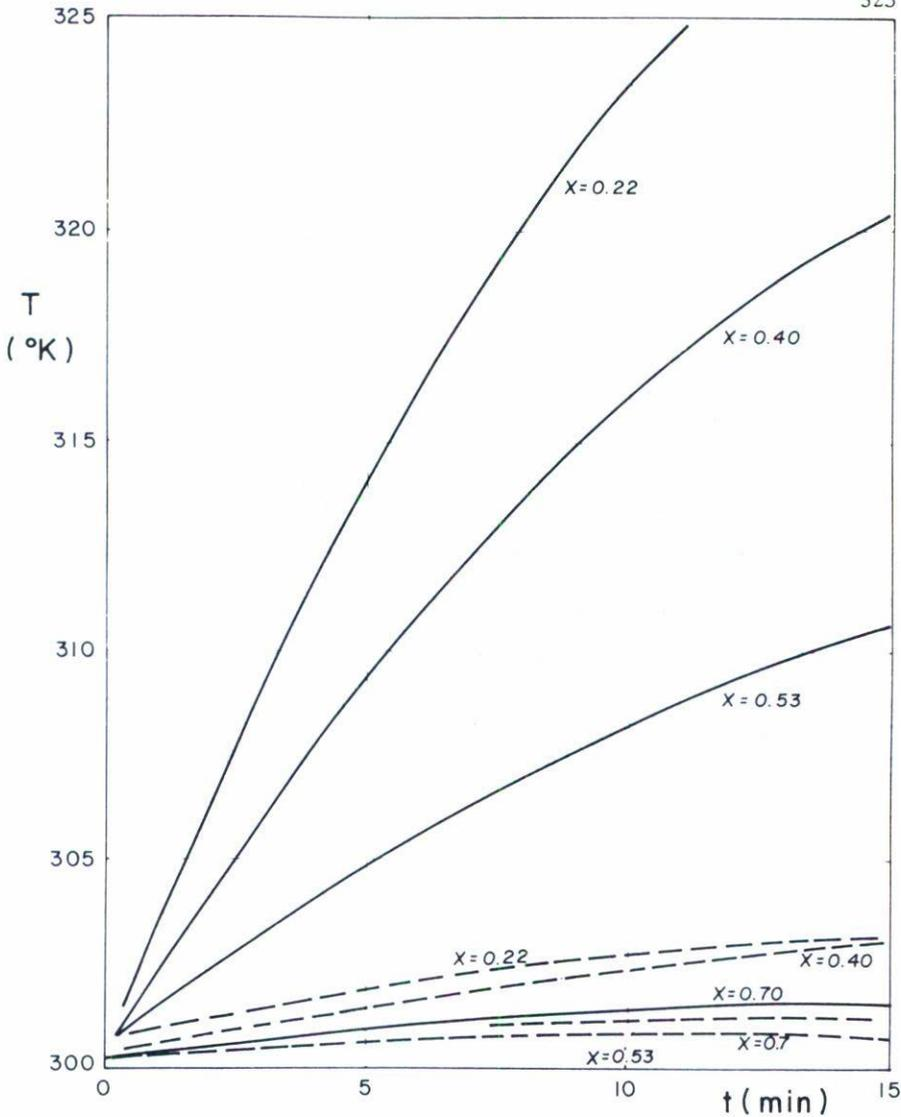
Fig. 5 Thermal behaviour of the samples in the Ni-Zn system. Continuous line, normal mode; broken line, burst mode.
