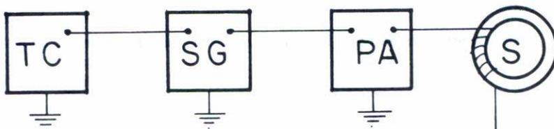
Fig. 3 Modification of the excitation signal in the burst system. TC-triggering circuit, SG-signal generator, PA-power amplifier, S-sample.
