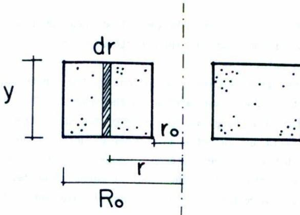
Fig. 2 Toroidal sample.  $r_o$  inner radius,  $R_o$  outer radius,  $y$  thickness,  $dr$  differential radius.
