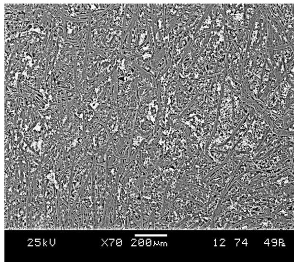
FIGURE 2. SEM image: paper sample without treatment.
