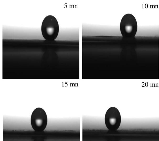
FIGURE 4. Water drop images for contact angle measurement.
