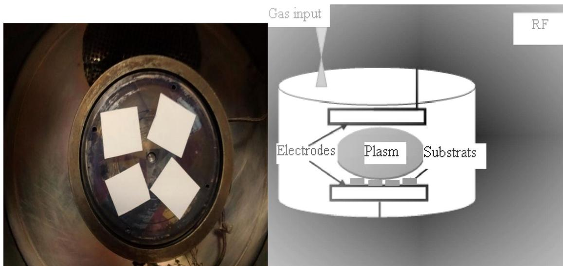
FIGURE 1. a) Substrates used for deposits. b) Scheme of a PECVD reactor chamber used for deposition.
