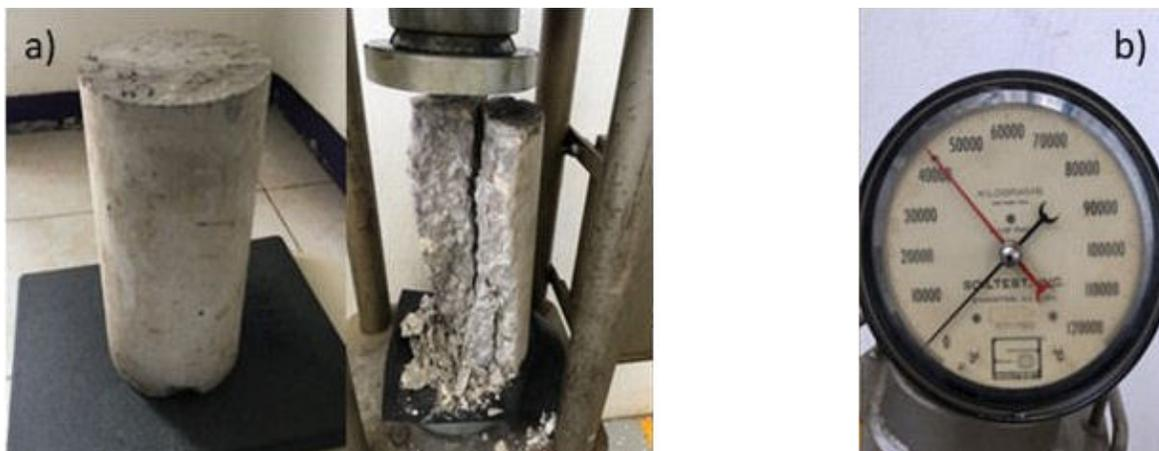
FIGURE 1. Compression test. a) Cylindrical concrete specimen. b) Tested specimen.
