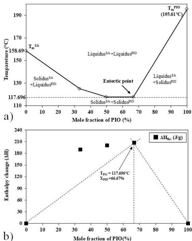
FIGURE 4. a) Binary phase diagram. b) Tamman's triangle graph of prepared eutectic formulation with PIO and SA.
