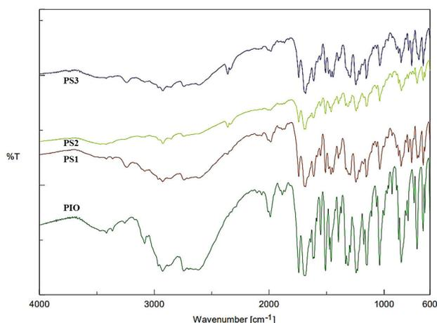
FIGURE 2. FTIR of PIO and PIO-SA eutectic formulations with different ratios for the determination of functional groups.
