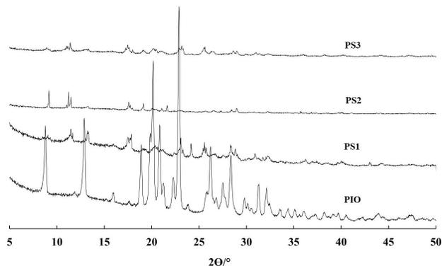
FIGURE 5. XRD pattern of PIO and PIO-SA eutectic formulation to check the crystallinity of raw PIO as well as prepared formulations.
