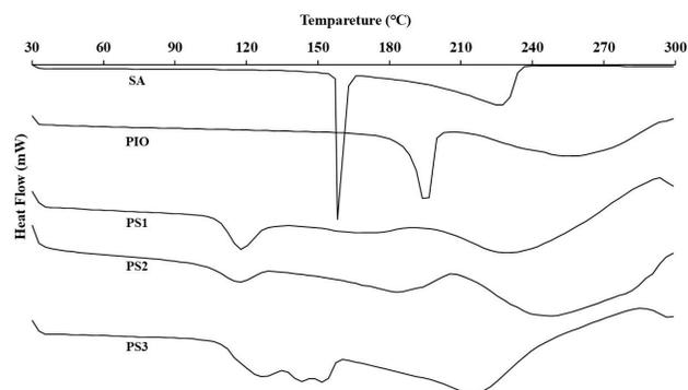
FIGURE 3. DSC thermogram of PIO, raw SA, and PIO-SA eutectic formulation (PS1, PS2, and PS3) to determine the melting endotherm.
