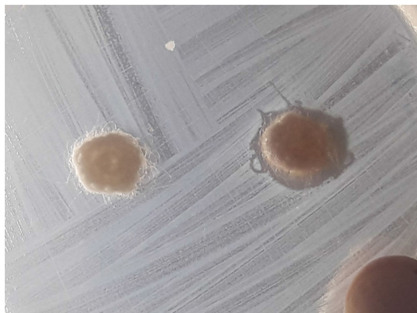
FIGURE 7. Antibacterial activity assay on Escherichia coli culture medium. The left sample corresponds to an unfunctionalized alpaca fiber, showing no inhibition of bacterial growth. The right sample shows a silver-functionalized alpaca fiber, evidenced by the clear inhibition zone surrounding the fiber. The background streaks indicate uniform bacterial growth across the medium.
