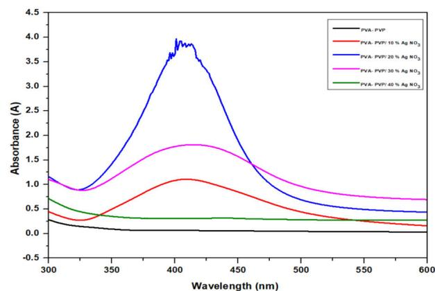
FIGURE 2. UV-VIS spectra of pure (PVA/PVP) with different concentration of  $\text{AgNO}_3$ .
