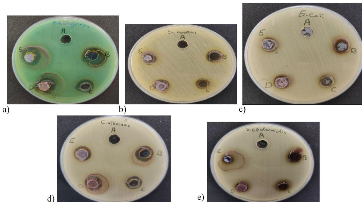
FIGURE 4. Inhibition zone (mm) of pure (PVA/PVP) at different concentrations of  $\text{AgNO}_3$ .
