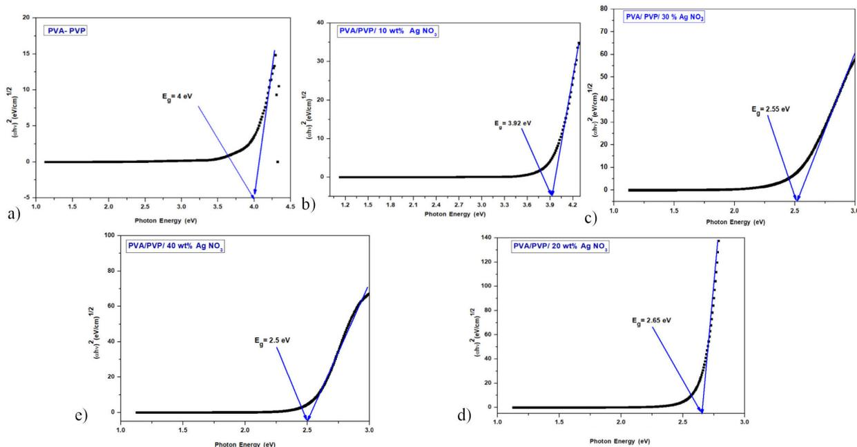
FIGURE 3. Direct band gap estimations of pure (PVA/PVP) with different concentration of  $\text{AgNO}_3$
