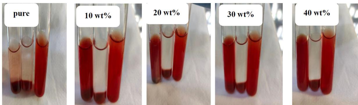
FIGURE 5. Toxicity of treatment with pure PVA/PVP with different concentrations of Ag NPs.
