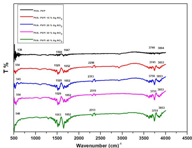
FIGURE 1. FTIR spectra of pure (PVA/PVP) with different concentration of  $\text{AgNO}_3$
