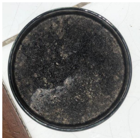
FIGURE 1. GO sample synthesized with \text{Fe}_3\text{O}_4 assistance.
