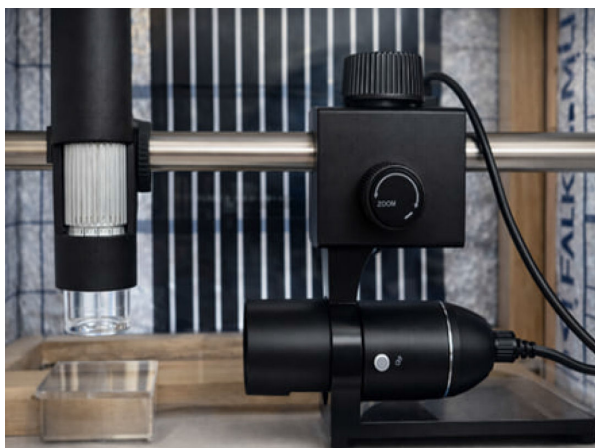
FIGURE 3. Digital USB microscope system used for acquiring droplet images during evaporation. This figure illustrates the imaging device only; quantitative geometric measurements were performed on calibrated digital images, as shown in Fig. 4.
