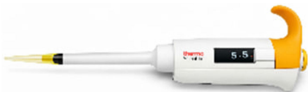
FIGURE 1. Automatic piston micropipette used for forming droplets and dispensing them onto the substrate surface (initial volume: 5.5 \mu\text{L} ).
