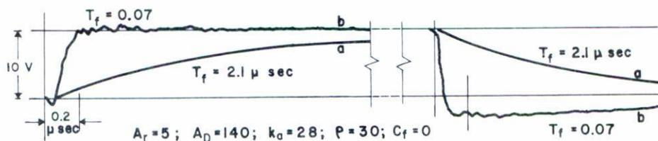
Fig. 6. Transient response of the a) non-compensated and b) correctly compensated amplifier shown in fig. 5. The experimental factor of figure of merit was  $\rho = 30$  with no feedback ( $C_f = 0$ ).
