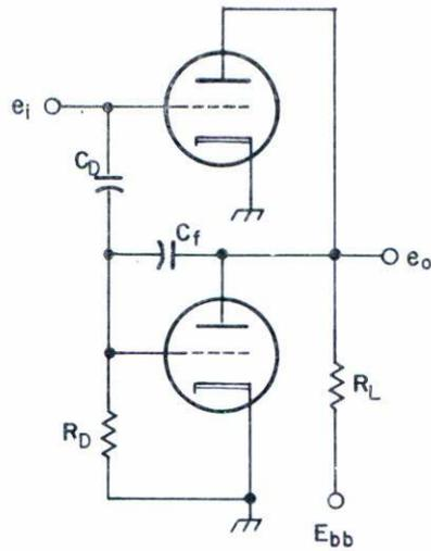
Fig. 3. The modified version of the elementary IDA unit with negative differentiated feedback through  $C_f$ .
