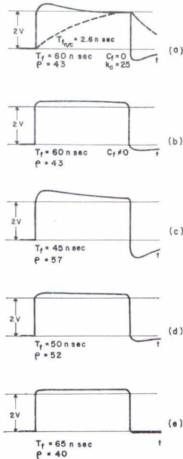
Fig. 7. Some experimental results with varying  $C_D$  and  $C_f$  and constant gains
