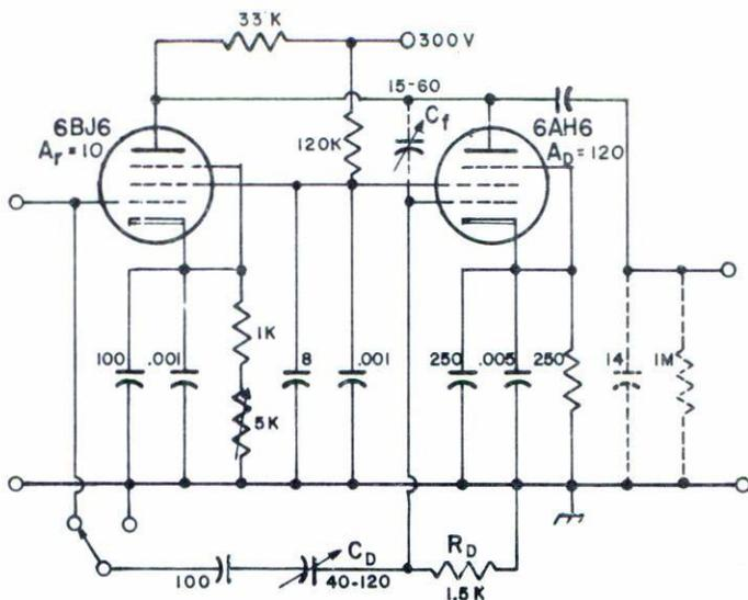
Fig. 5. Diagramme of the experimental amplifier constructed to verify the action of the differentiator  $R_D - C_D$  and of the capacitor  $C_f$  for the cancellation of the overshoot.
