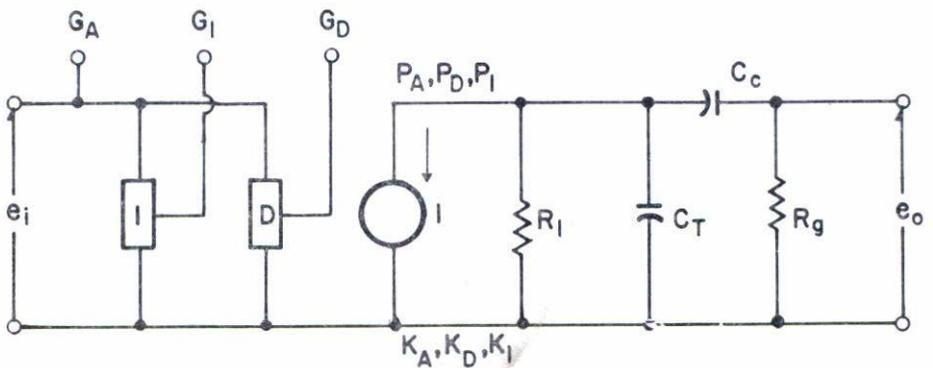
Fig. 2. A proposed equivalent plate circuit of the IDA unit. The  $C_{gp}$  capacitance was omitted.
