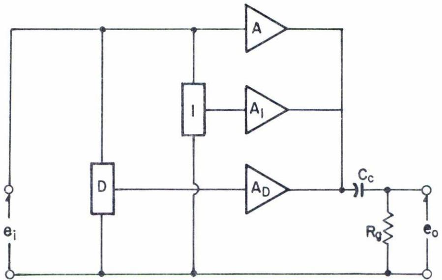
Fig. 1. Block diagramme of IDA unit. D and I are the differentiator and integrator, respectively; A,  $A_D$  and  $A_I$  are conventional amplifiers.
