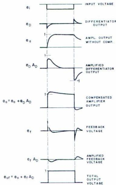
Fig. 4. A qualitative representation of the operation of the elementary IDA unit with negative feedback. The low-frequency response is assumed flat.
