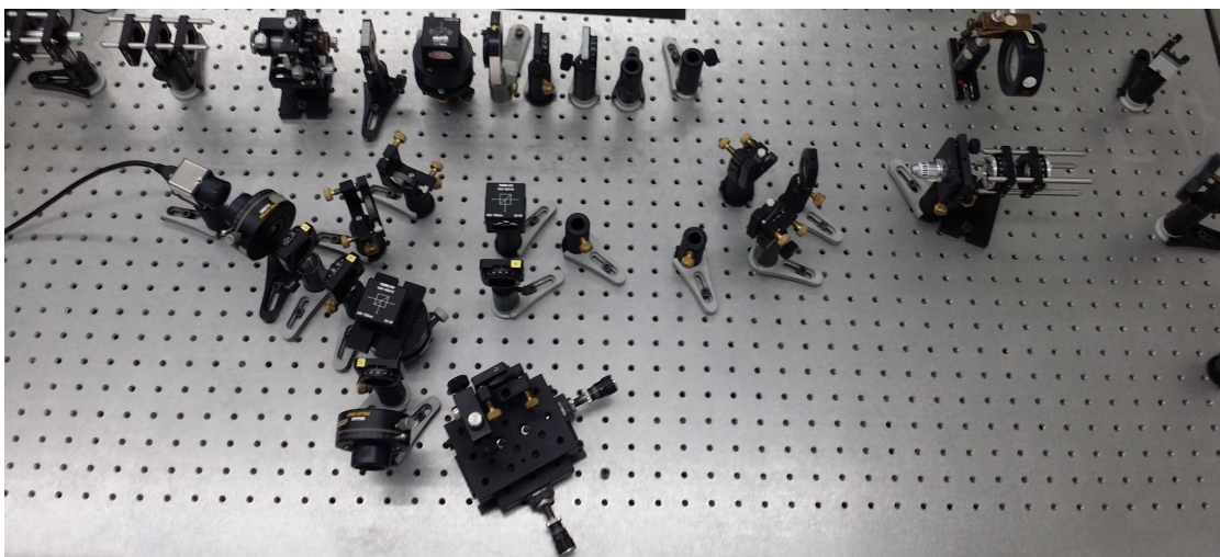
FIGURE 4. Experimental setup proposed here to determine the Mueller matrix using a single azimuthally polarized beam of light @532 nm (following Ref. 13).
