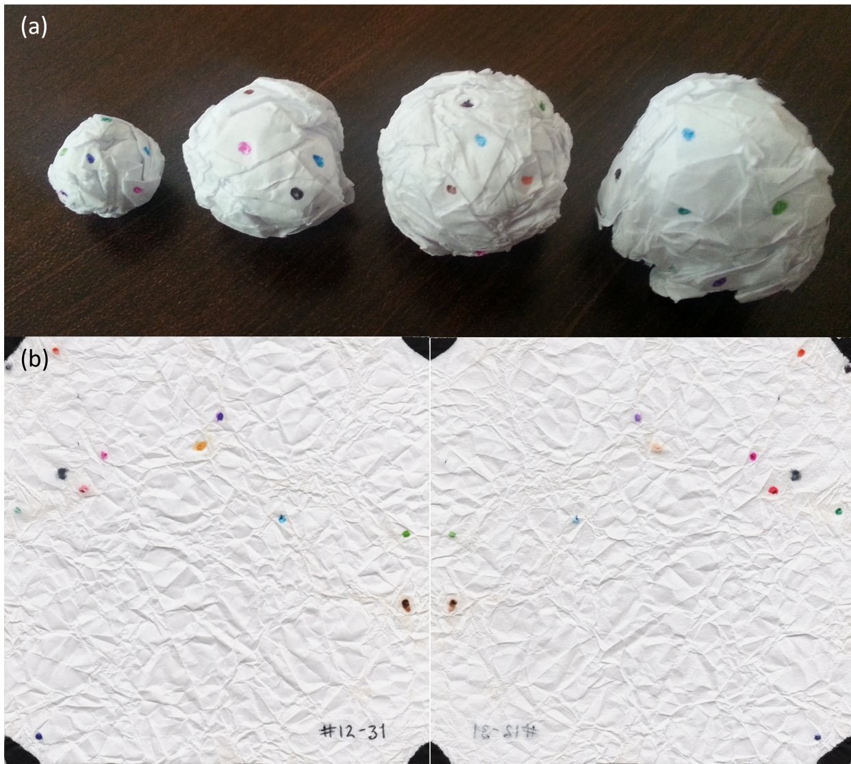
FIGURE 1. Copy paper type employed in the experiment. (a) Relaxed strain crumpled configuration and (b) Digitized sheet after being unfolded and flattened. The black corners were a guide to de eye.
