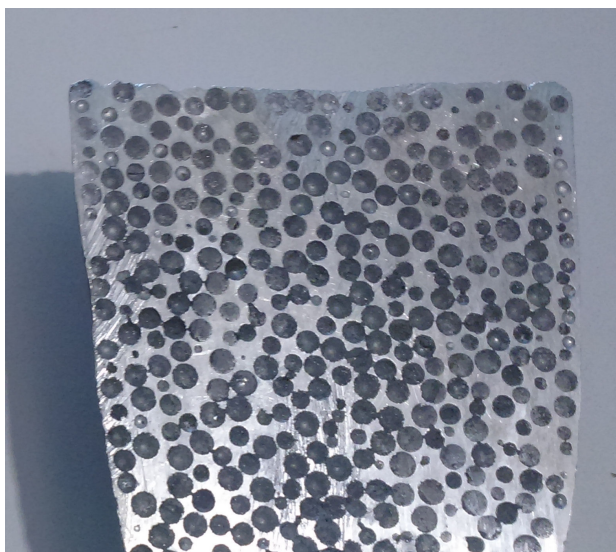
FIGURE 1. A face of borosilicate spheres - Zn22Al2Cu composite. M, matrix.
