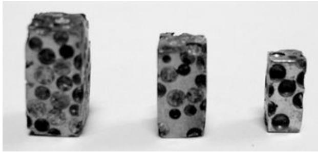
FIGURE 2. Samples of the three sizes used for the compression test.
