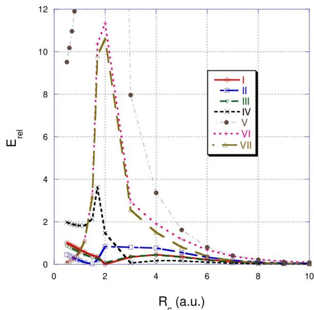
FIGURE 1. Relative percentage error in the ground state energy of CHA produced by the seven different trial wavefunctions as a function of the confinement radius  $R_c$ . The wavefunction V gives the mayor errors. Whereas the wavefunctions V and VI give the lowest errors for the strong confinement.
