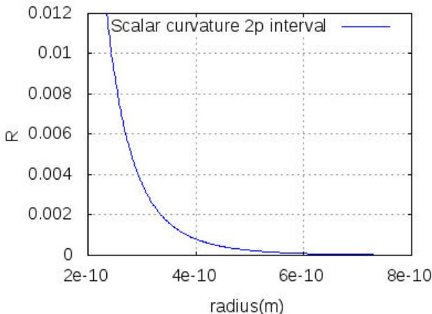
FIGURE 2. Curvature as a function of radius in the maximal probability interval.
