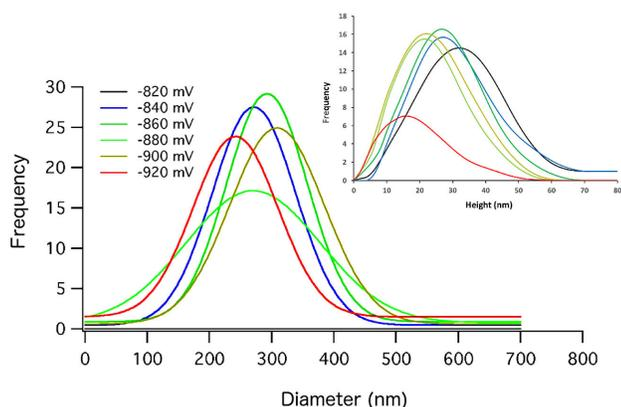
FIGURE 3. Frequency histogram of the diameter and height (inset) of the clusters at different formation potentials.
