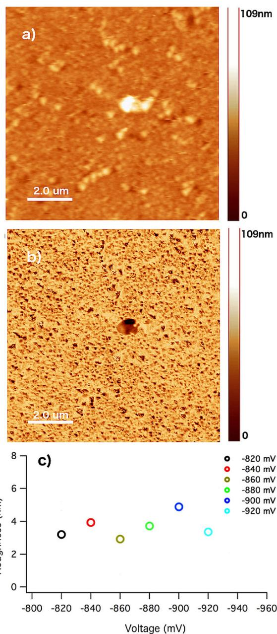
FIGURE 2. a) AFM and b) MFM images of the Au surface after Co deposition. c) corresponds to the roughness values at different formation potentials. Image sizes are  $10 \mu\text{m} \times 10 \mu\text{m}$ .
