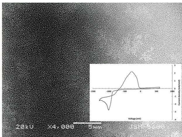
FIGURE 1. SEM image of the gold surface after Co electrodeposition. The inset corresponds to the Cyclic voltammetry plot for the cobalt deposition onto Au.
