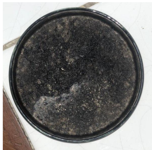
FIGURE 1. GO sample synthesized with \text{Fe}_3\text{O}_4 assistance.
