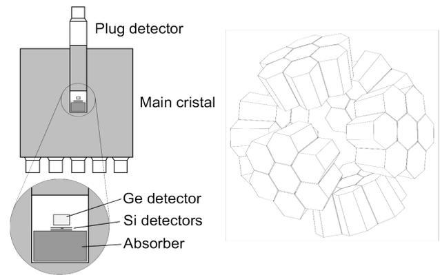
FIGURE 2. The two different experimental setups used in the GSI experiments. Right: cube of 6 cluster detectors (CLUSTER CUBE). Left: schematic view of the GSI Total Absorption Spectrometer and its ancillary detectors.
