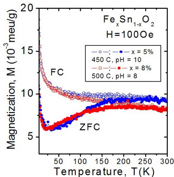
FIGURE 3. Zero-field-cooled (ZFC) and field-cooled (FC) curves as a function of the temperature ( $T$ ) obtained at  $H=100$  Oe for the Fe-doped  $\text{SnO}_2$  nanoparticles.
