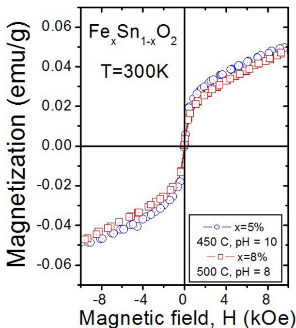
FIGURE 4. Magnetization ( $M$ ) as a function of the magnetic field ( $H$ ) obtained at 300 K for the samples indicated in the figure.
