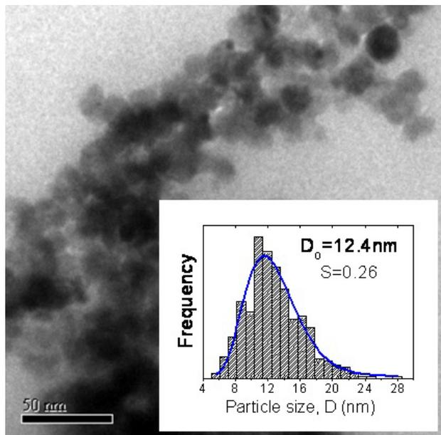
FIGURE 2. TEM image obtained for the Fe-doped  $\text{SnO}_2$  nanoparticles with 8 mol% Fe (pH=8). In the inset is shown the histogram mounted as described in the text and modeled by the log-normal function.
