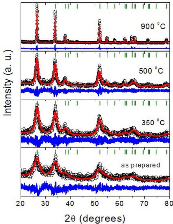
FIGURE 1. XRD patterns of the Fe-doped SnO<sub>2</sub> with 8 mol% (pH=8). The thermal treatments were carried out for 1h in the temperatures showed in each plot.
